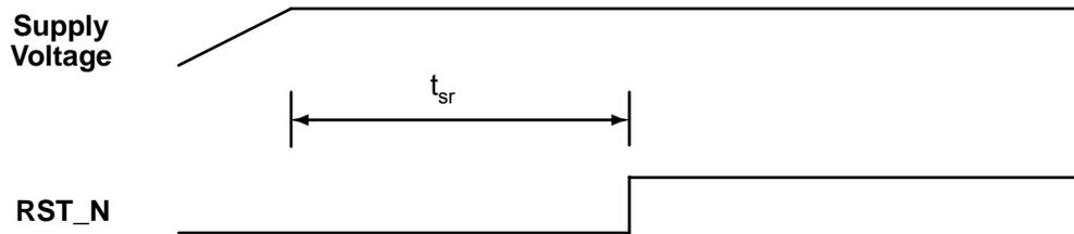
**Figure 9. Reset Timing**
