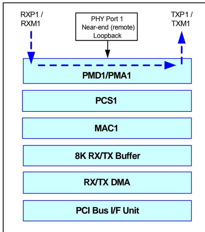
**Figure 6. Port 1 Near-End (Remote) Loopback Path**
