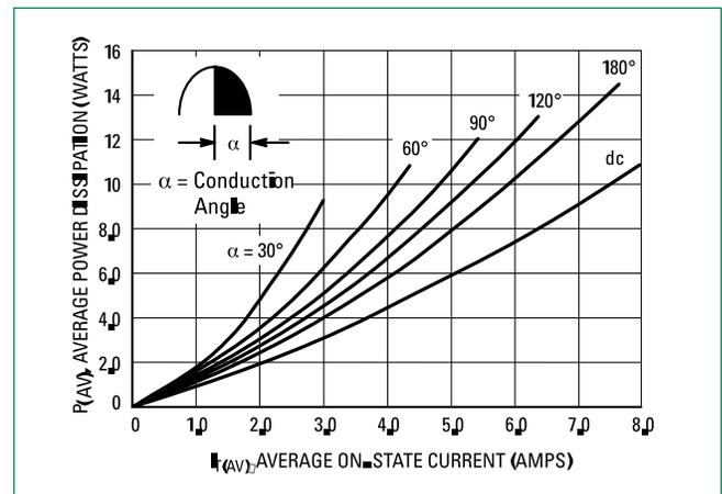
**Figure 3. On-State Characteristics**
