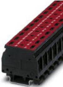
Modular double terminal block with gas-filled surge arrester as coarse protection between both levels, nominal voltage: 250 V AC, for mounting on NS 32 or NS 35/7.5, closed housing, terminal width: 15.5 mm, terminal height: 45.5 mm
