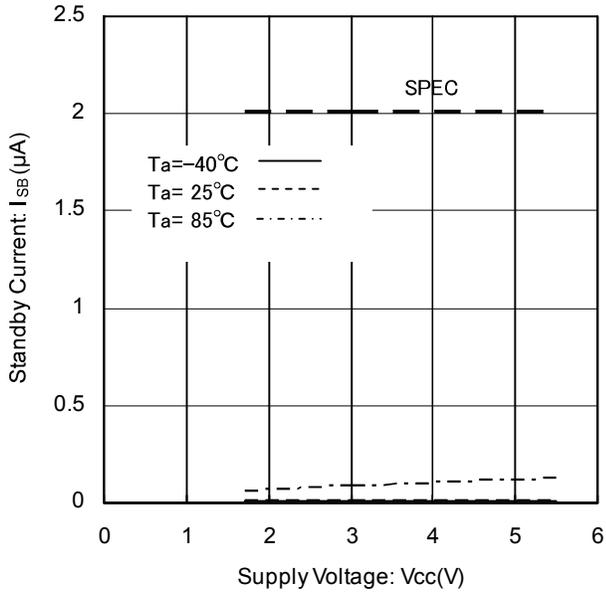
Figure 12. Standby Current vs Supply Voltage
