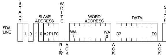
Figure 35. Byte Write Cycle
