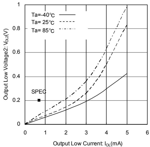
Figure 7. Output Low Voltage<sub>2</sub> vs Output Low Current (Vcc=1.6V)
