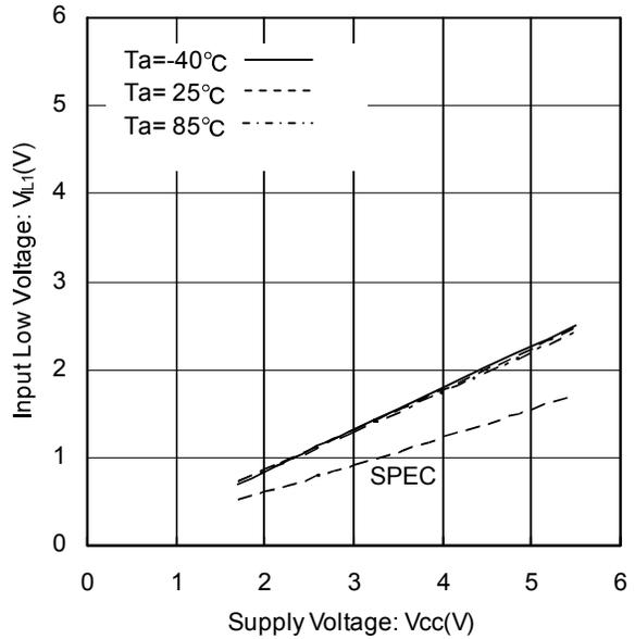
Figure 5. Input Low Voltage<sub>1,2</sub> vs Supply Voltage (A2, SCL, SDA, WP)
