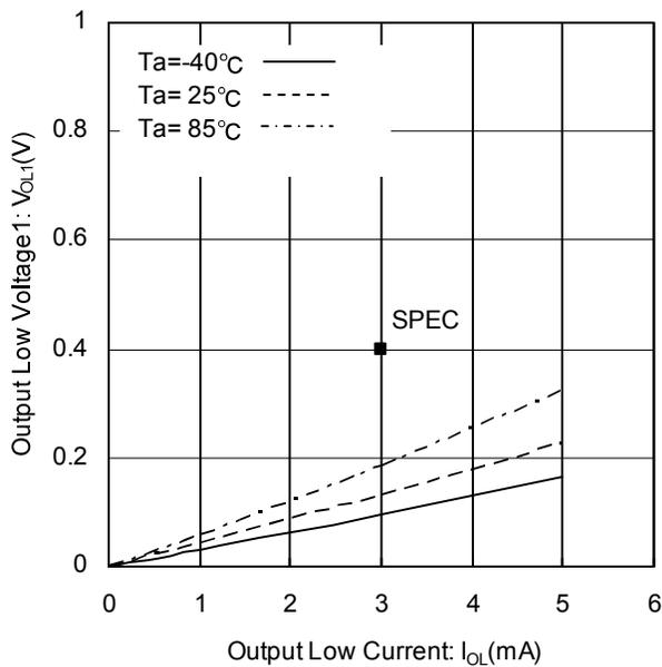
Figure 6. Output Low Voltage<sub>1</sub> vs Output Low Current (Vcc=2.5V)
