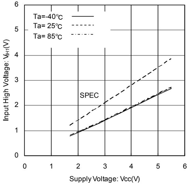
Figure 4. Input High Voltage<sub>1,2</sub> vs Supply Voltage (A2, SCL, SDA, WP)
