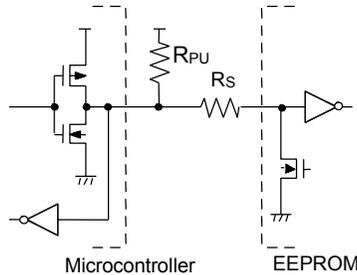
Figure 45. I/O Circuit Diagram
