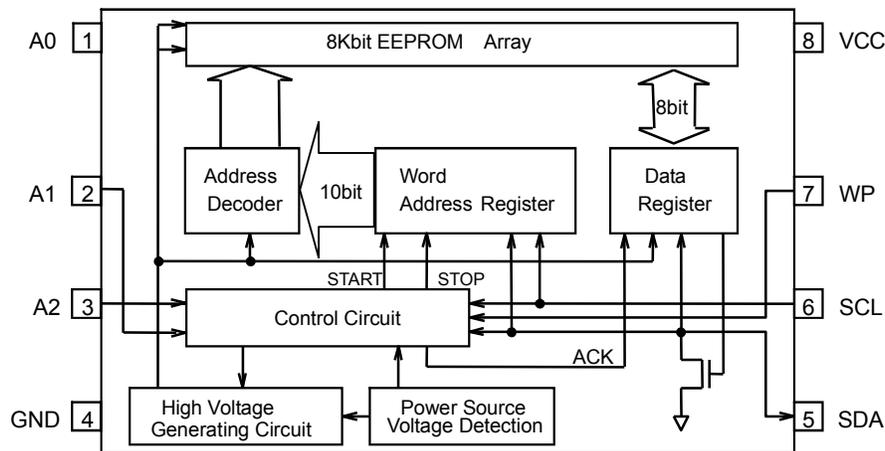
Figure 3. Block Diagram
