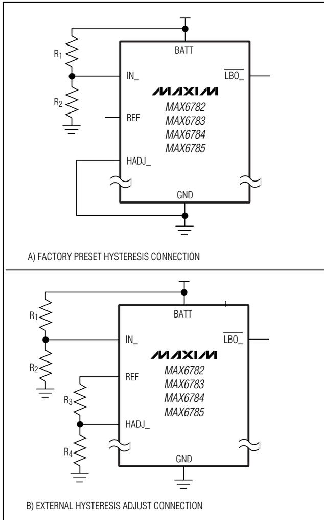
Figure 6. Internal Preset or Externally Adjusted Hysteresis Connection
