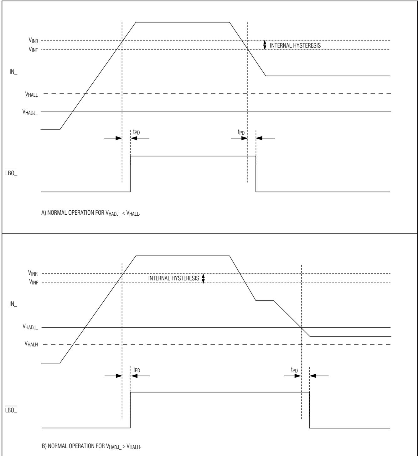
Figure 4. MAX6782-MAX6785 Timing
