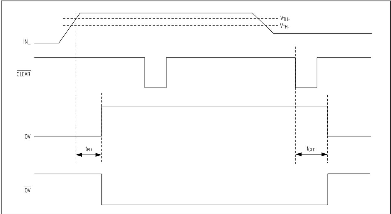
Figure 5. MAX6789/MAX6790 Timing
