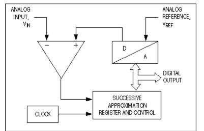
Figure 2. Typical successive-approximation ADCs consist of a single DAC, a comparator, and a successive-approximation register (SAR), plus a clock and logic control.
