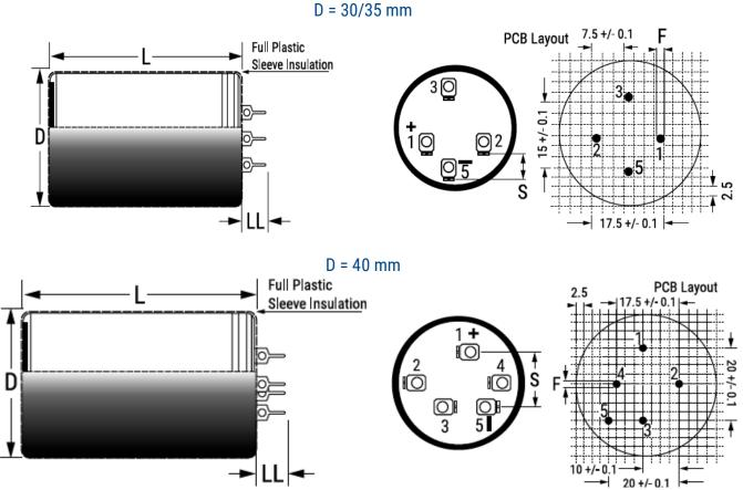
Connections: Hole 1 represents +ve. Hole 5 Represents -ve. Terminals 2,3, and 4 may be at negative terminal potential due to the presence of electrolyte. They are intended for mechanical connections only. It is recommended that they are soldered to the printed cicuit board. Additional dummy pins are provided for stability. Note that the case and dummy pins may be at negavitve terminal potential
