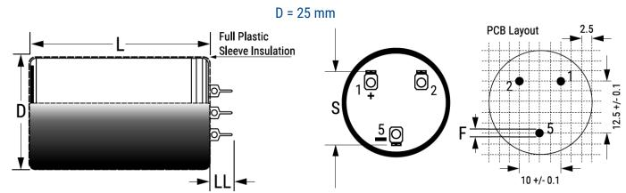
Connections: Hole 1 represents +ve. Hole 5 Represents -ve. Terminals 2,3, and 4 may be at negative terminal potential due to the presence of electrolyte. They are intended for mechanical connections only. It is recommended that they are soldered to the printed cicuit board. Additional dummy pins are provided for stability. Note that the case and dummy pins may be at negavtive terminal potential
