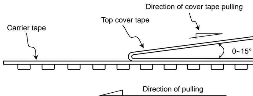
3-2. Carrier tape shall be flexible enough to be wound around a minimum radius of 30mm with components in tape.
