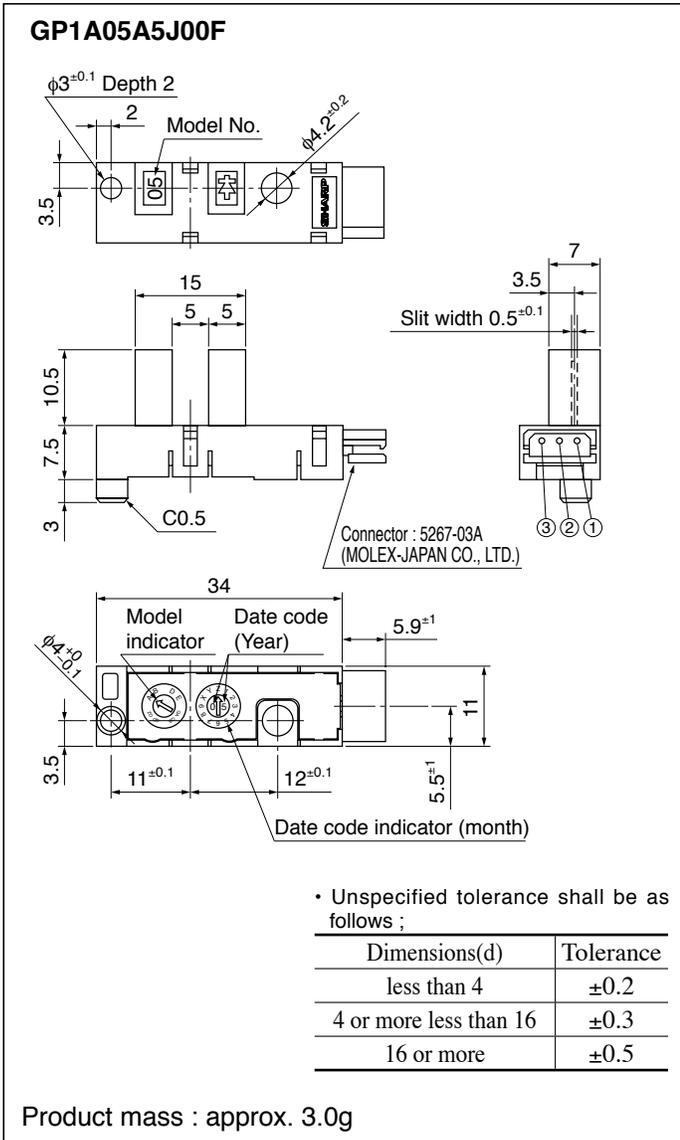
Connector terminal plating material : Sn
