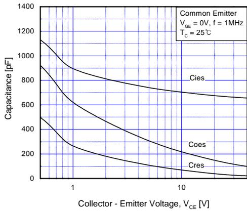
**Fig 7. Capacitance Characteristics**
