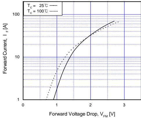
Fig 18. Forward Characteristics
