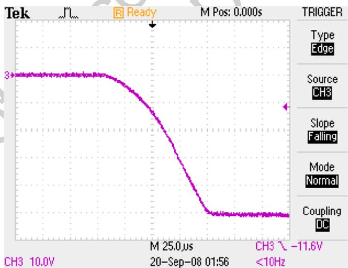
Figure 5. Turn-On Waveform—V<sub>port</sub> Relative to GND
