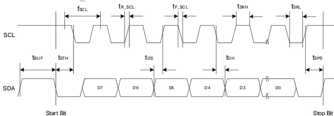
**Figure 1. I<sup>2</sup>C Timing Diagram**
