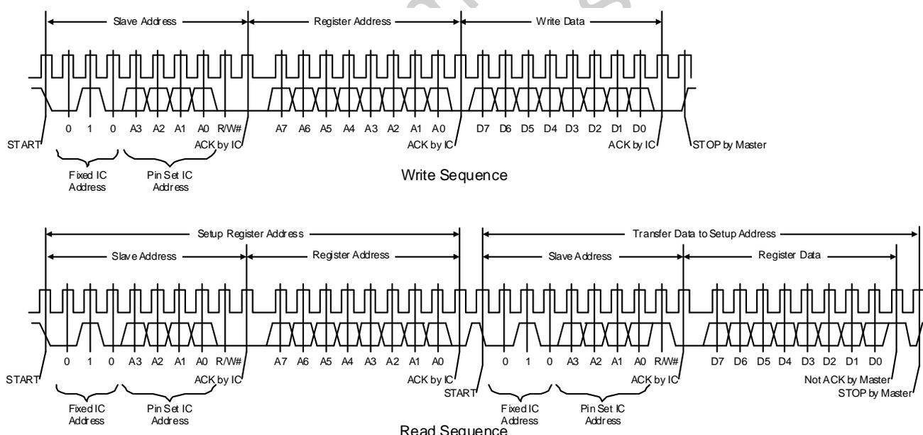
**Figure 6. Typical I<sup>2</sup>C Bus Transactions**
