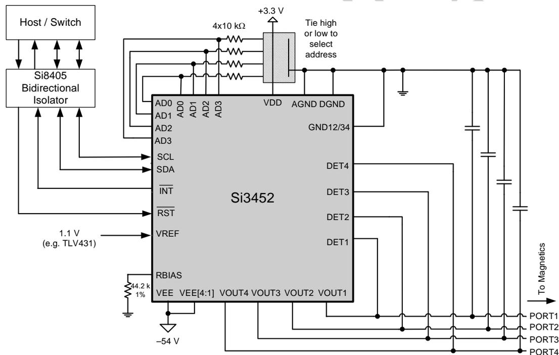
Figure 3. 4-Port Application Diagram Using dV/dt Disconnect and I<sup>2</sup>C Host Interface
