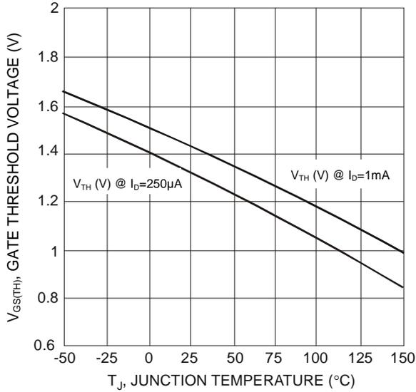
Fig. 7 Gate Threshold Variation vs. Junction Temperature
