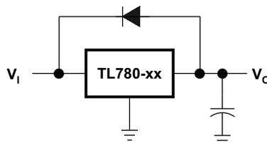
**Figure 5. Reverse-Bias-Protection Circuit**
