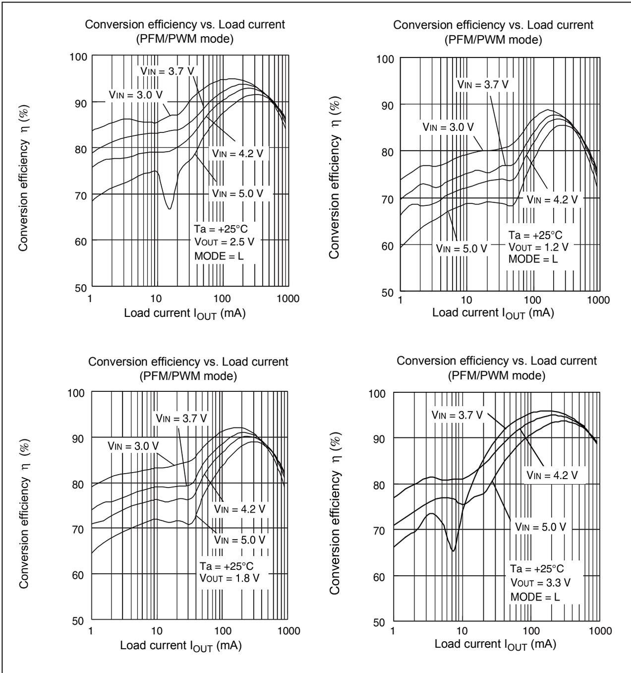
Conversion efficiency vs. Load current
