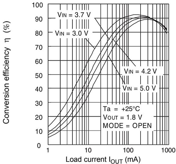
Conversion efficiency vs. Load current
