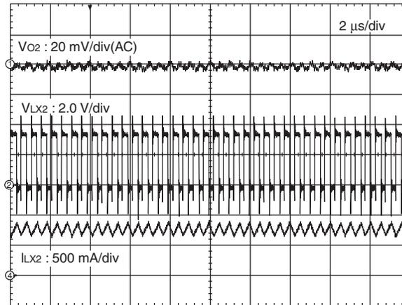
V<sub>IN</sub> = 3.7 V, V<sub>O2</sub> = 1.8 V, I<sub>o2</sub> = -800 mA, MODE = L, T<sub>a</sub> = +25 °C
