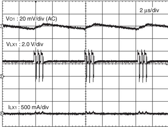
V<sub>IN</sub> = 3.7 V, I<sub>o1</sub> = -5 mA, V<sub>O1</sub> = 2.5 V, MODE = L, T<sub>a</sub> = +25 °C
