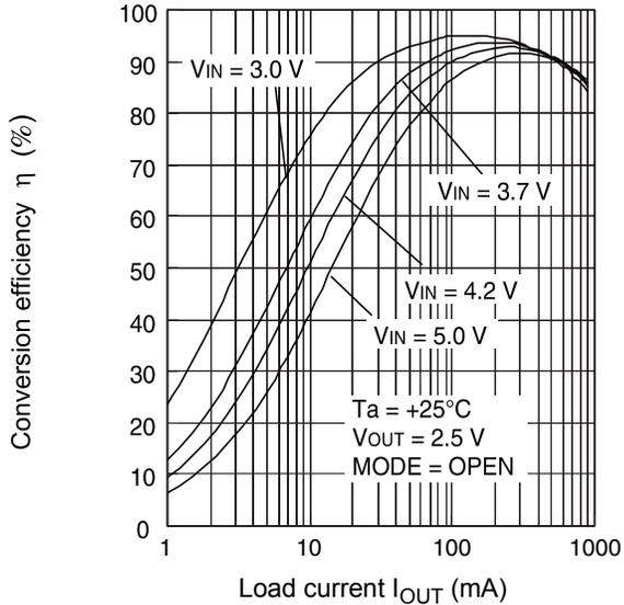
Conversion efficiency vs. Load current
