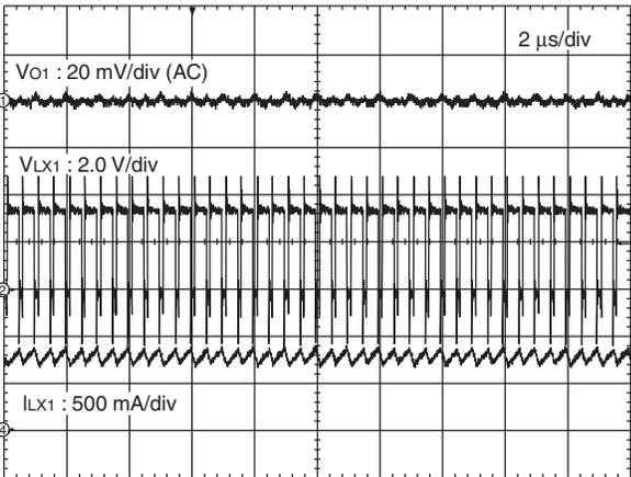
V<sub>IN</sub> = 3.7 V, V<sub>O1</sub> = 2.5 V, I<sub>o1</sub> = -800 mA, MODE = L, T<sub>a</sub> = +25 °C
