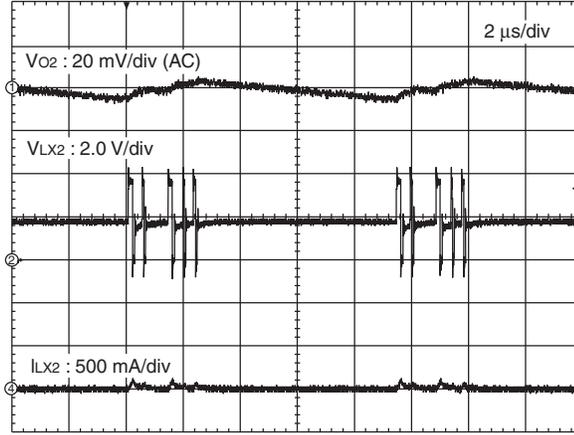
V<sub>IN</sub> = 3.7 V, I<sub>o2</sub> = -5 mA, V<sub>O2</sub> = 1.8 V, MODE = L, T<sub>a</sub> = +25 °C
