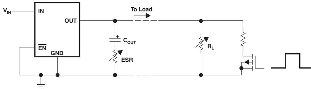
Figure 29. Test Circuit for Typical Regions of Stability
