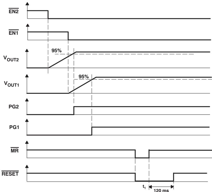
NOTES: A.  $t_1$ : Time at which  $V_{IN}$  is greater than  $V_{UVLO}$  and  $\overline{MR}$  is logic high.
