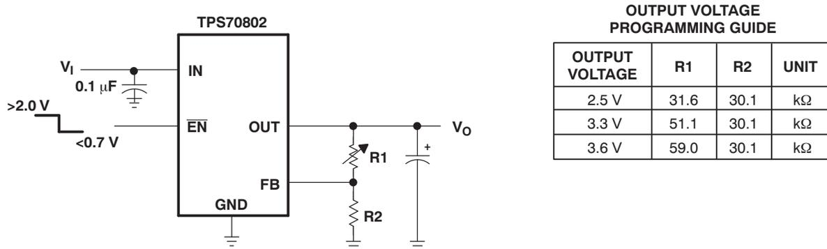
Figure 40. TPS70802 Adjustable LDO Regulator Programming
