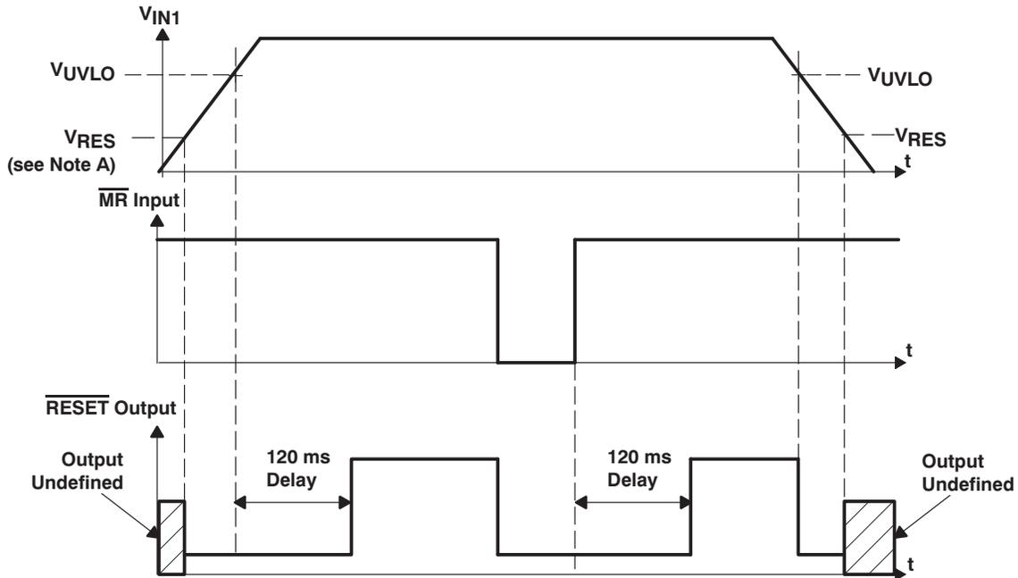
NOTE A:  $V_{RES}$  is the minimum input voltage for a valid  $\overline{RESET}$ . The symbol  $V_{RES}$  is not currently listed within EIA or JEDEC standards for semiconductor symbology.
