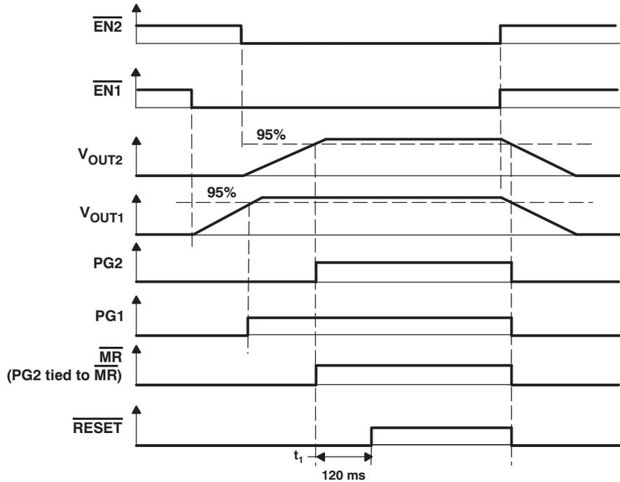
NOTES: A.  $t_1$ : Time at which  $V_{IN}$  is greater than  $V_{UVLO}$  and  $\overline{MR}$  is logic high.
