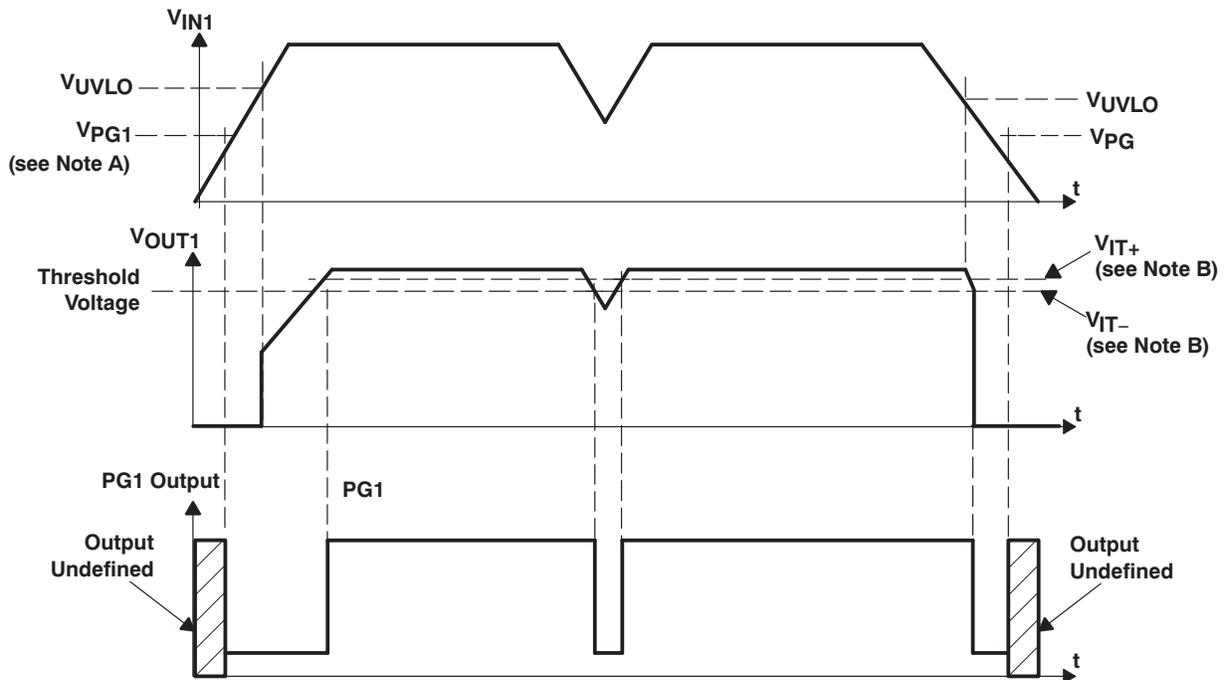
NOTES A:  $V_{PG1}$  is the minimum input voltage for a valid PG. The symbol  $V_{PG1}$  is not currently listed within EIA or JEDEC standards for semiconductor symbology.
