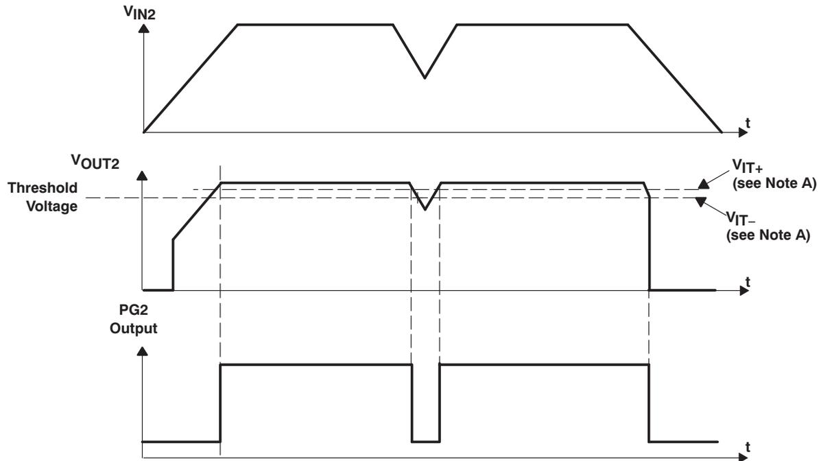
NOTE A:  $V_{IT-}$  trip voltage is typically 5% lower than the output voltage ( $95\%V_O$ ).  $V_{IT-}$  to  $V_{IT+}$  is the hysteresis voltage.
