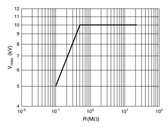
**HVR37** For 5 % tolerance  $\Delta R \pm (4.0 \% R + 0.1 \Omega)$  For 1 % tolerance  $\Delta R \pm (2.0 \% R + 0.1 \Omega)$
