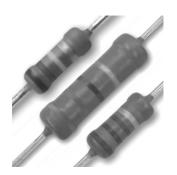
A homogenous film of metal alloy is deposited on a high grade ceramic body. After a helical groove has been cut in the resistive layer, tinned electrolytic copper wires are welded to the end-caps. The resistors are coated with a blue, non-flammable lacquer, which provides electrical, mechanical, and climatic protection.
