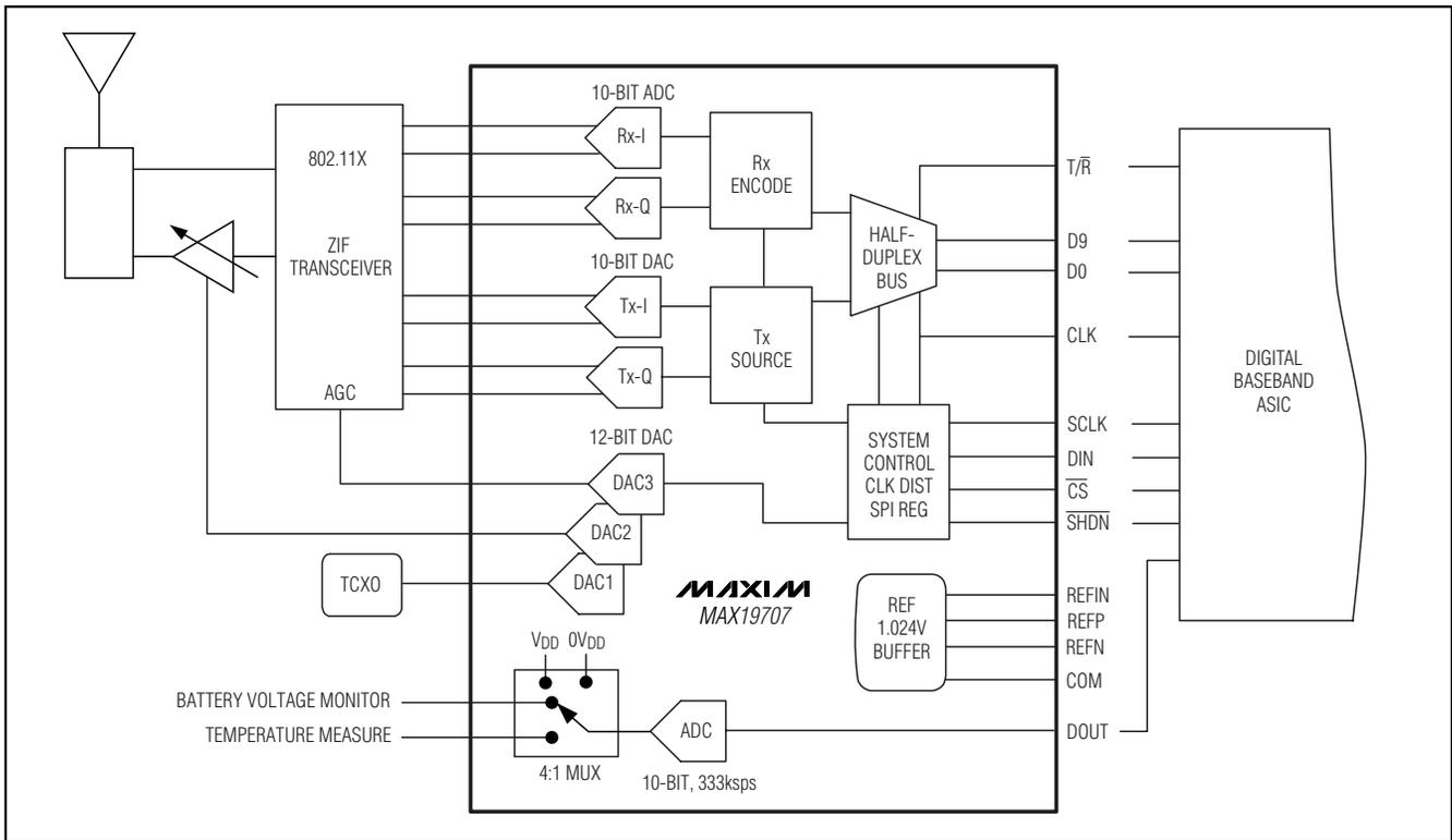
Figure 12. Typical Application Circuit for 802.11 Radio
