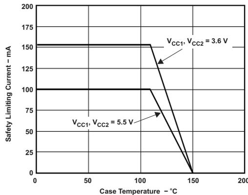
**Figure 8. θ<sub>JC</sub> Thermal Derating Curve Per IEC 60747-5-2**
