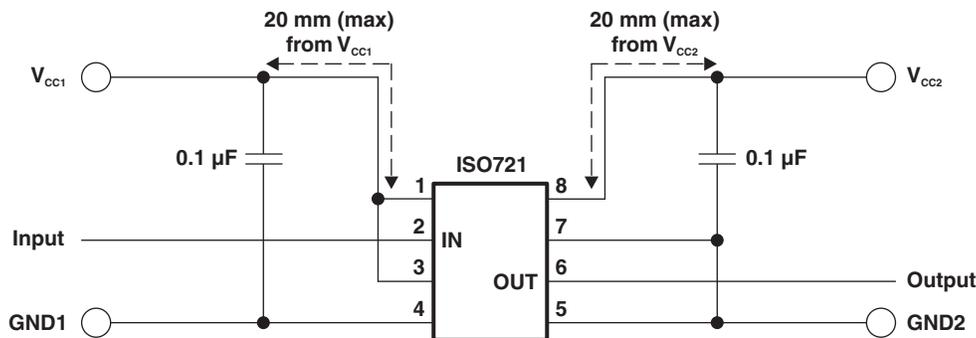
Figure 18. Basic Application Circuit
