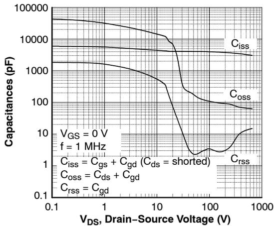
Figure 5. Capacitance Characteristics
