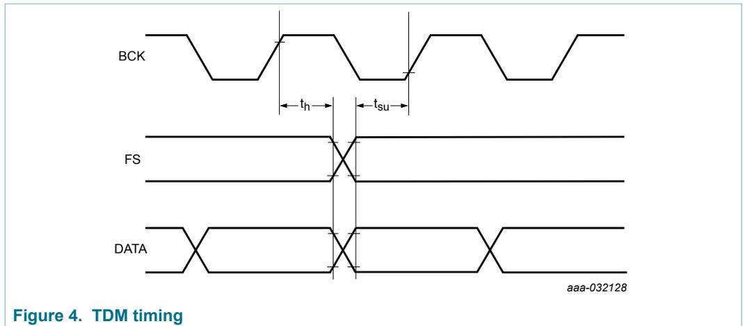
Figure 4. TDM timing
