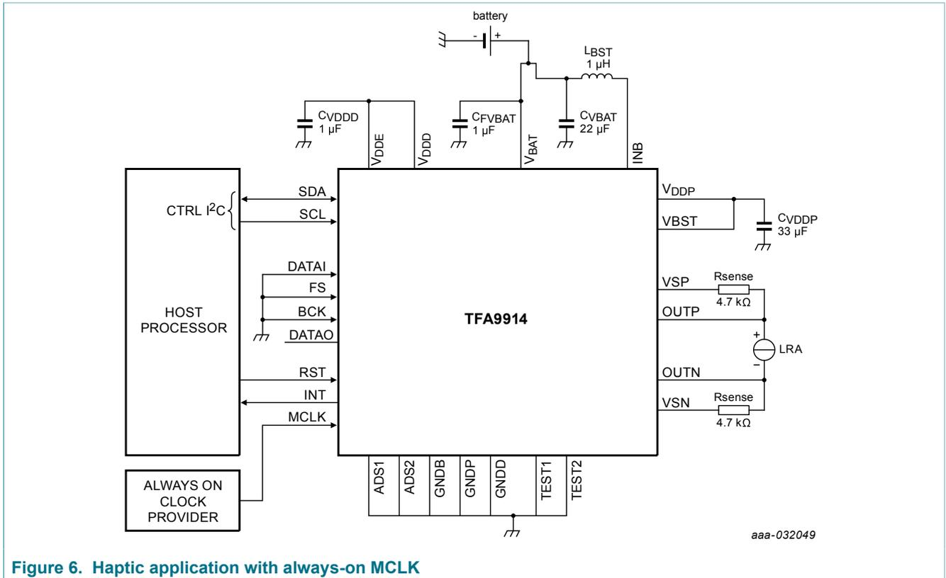
Figure 6. Haptic application with always-on MCLK
