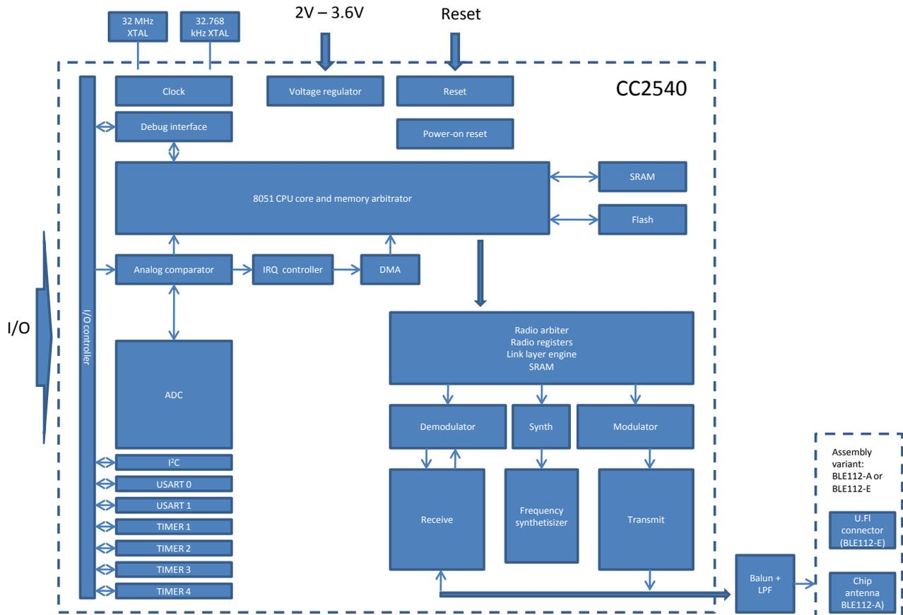
Figure 17: Simplified block diagram of BLE113
