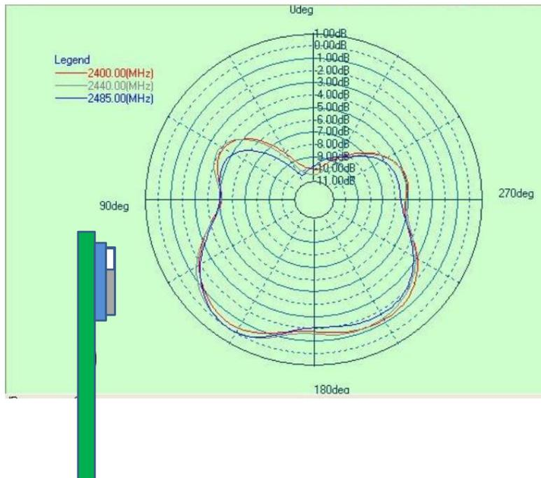
Figure 5: Radiation pattern of BLE113, front view
