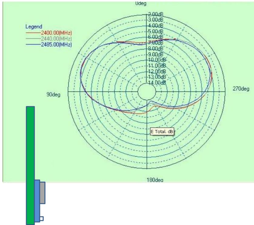
Figure 6: Radiation pattern of BLE113, side view
