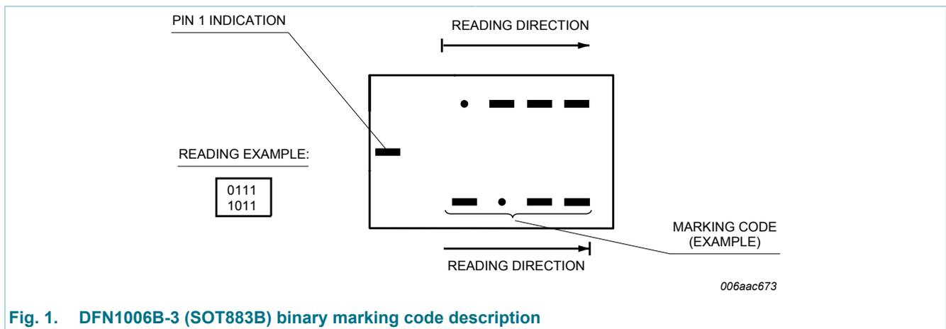
Fig. 1. DFN1006B-3 (SOT883B) binary marking code description
