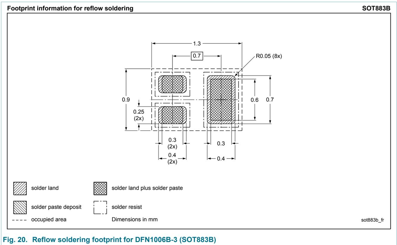
Fig. 20. Reflow soldering footprint for DFN1006B-3 (SOT883B)
