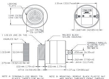
NOTE A: TERMINALS-.032 BRASS TIN PLATED, TAPPED FOR #6-32 SCREW. TWO #6-32 NICKEL PLATED BRASS SCREWS INCLUBED. WILL ACCEPT 1/4' GUICK CONNECT.
