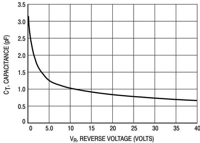
Figure 3. Typical Capacitance
