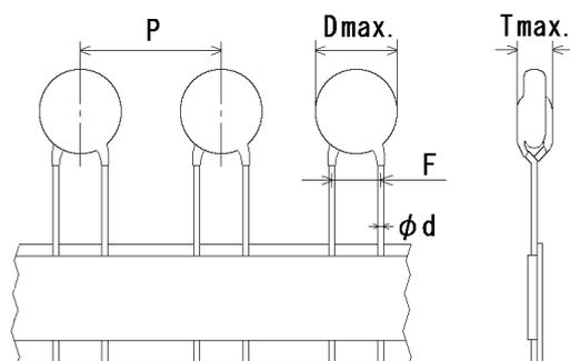
Note) The mark '\*' of Lead Style differ from lead spacing(F) and lead diameter(d) and pitch of component(P).
