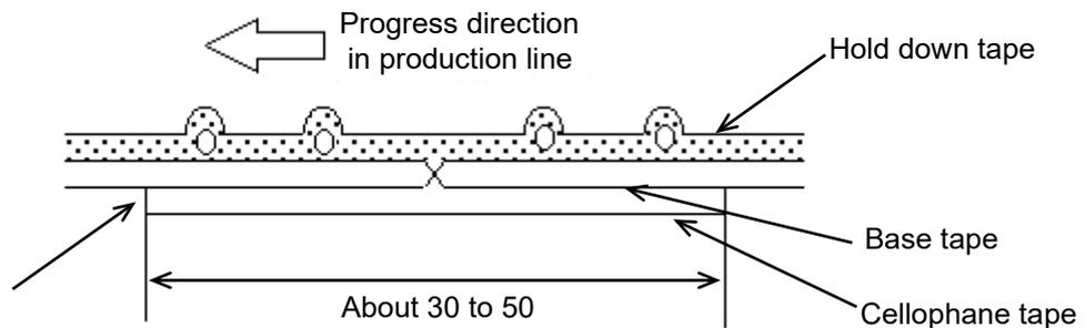
No lifting for the direction of progressing
