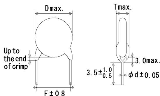
Note) The mark '\*' of Lead Style differ from lead spacing(F) and lead diameter(d).
