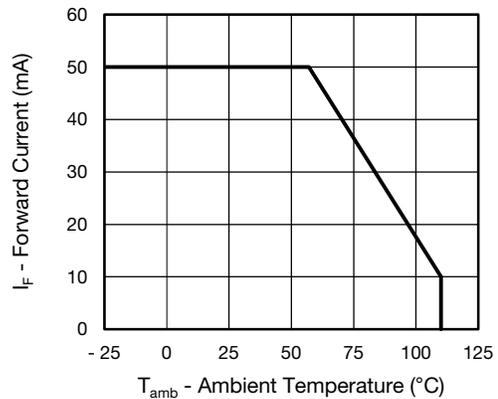
Fig. 2 - Forward Current vs. Ambient Temperature
