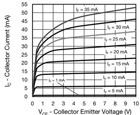
Fig. 6 - Collector Current vs. Collector Emitter Voltage
