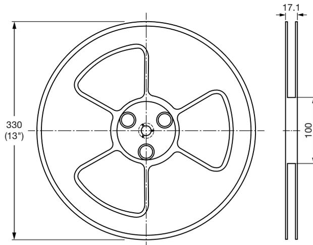
Fig. 17 - Reel Dimensions (3000 units per reel)
