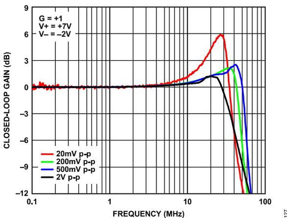
Figure 25. Frequency Response for Various Output Voltages
