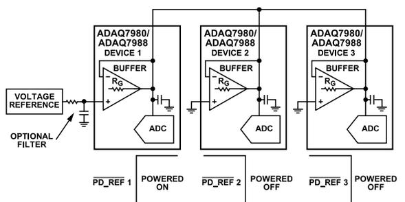
Figure 69. Reference Configuration for Multiple ADAQ7980/ADAQ7988 Devices
