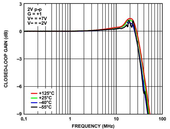
Figure 22. Large Signal Frequency Response for Various Temperatures
