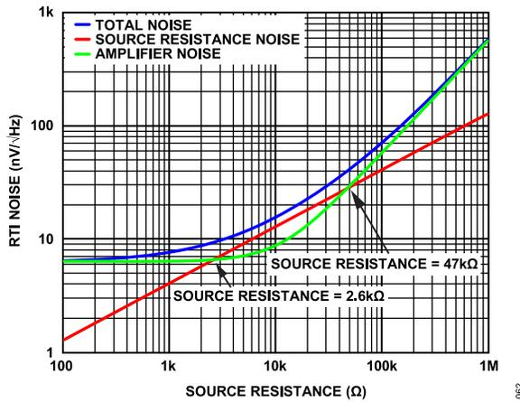
Figure 59. RTI Noise vs. Source Resistance
