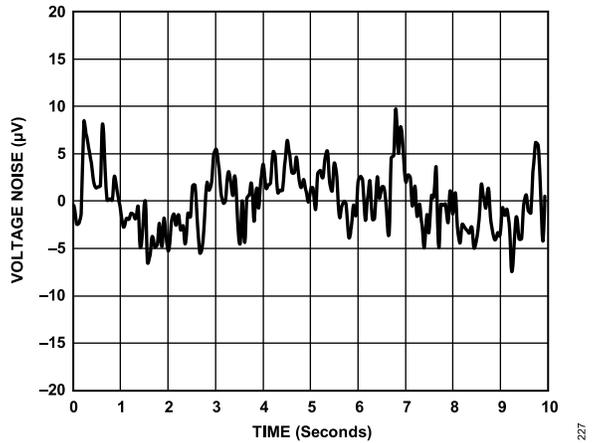
Figure 27. 0.1 Hz to 10 Hz Voltage Noise
