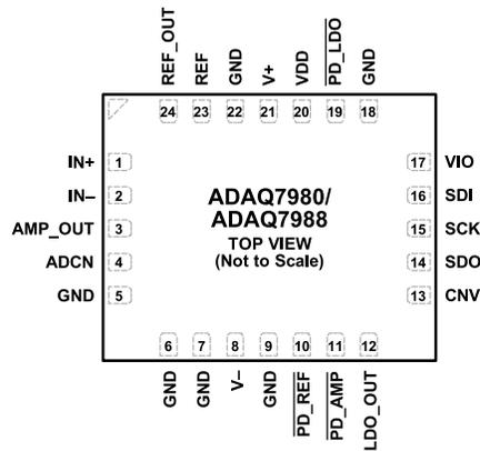
Figure 4. Pin Configuration
