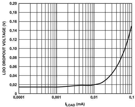
Figure 49. LDO Dropout Voltage vs. Load Current (I<sub>LOAD</sub>), LDO\_OUT = 2.5 V
