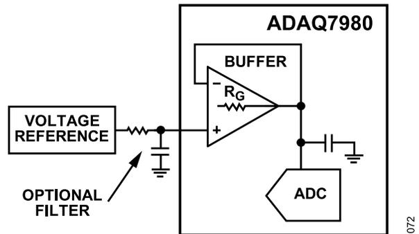
Figure 67. Voltage Reference with RC Filtering
