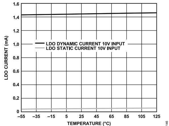
Figure 43. LDO Current vs. Temperature for Various Supplies
