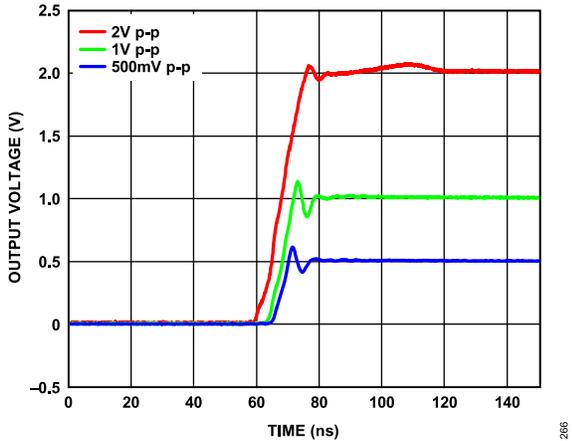
Figure 65. Step Response with Selected Output Steps
