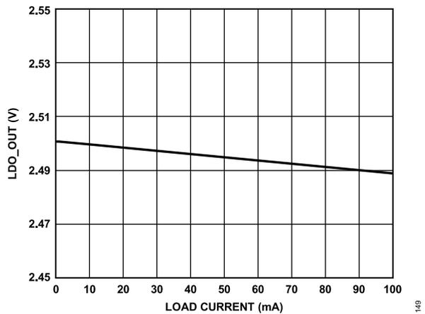
Figure 46. Output Voltage (LDO\_OUT) vs. Load Current ( $I_{LOAD}$ )
