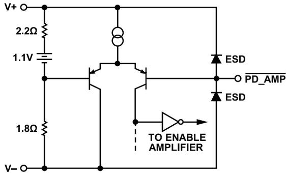
Figure 61. Shutdown Circuit
