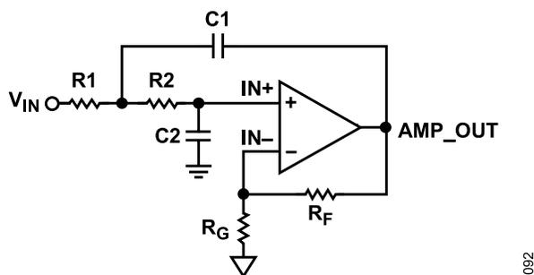
Figure 87. Schematic of a Second-Order, Low-Pass Active Filter
