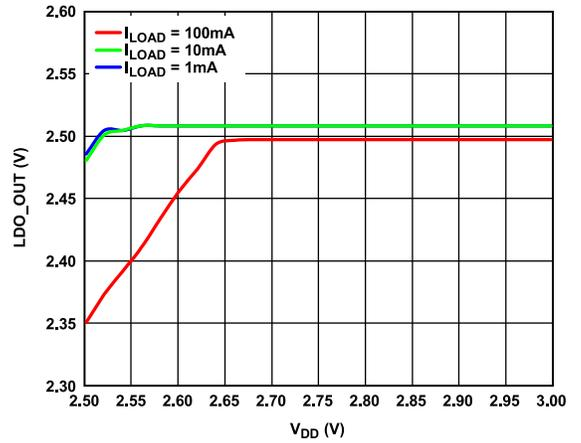
Figure 50. LDO\_OUT vs. V<sub>DD</sub> in Dropout, LDO\_OUT = 2.5 V
