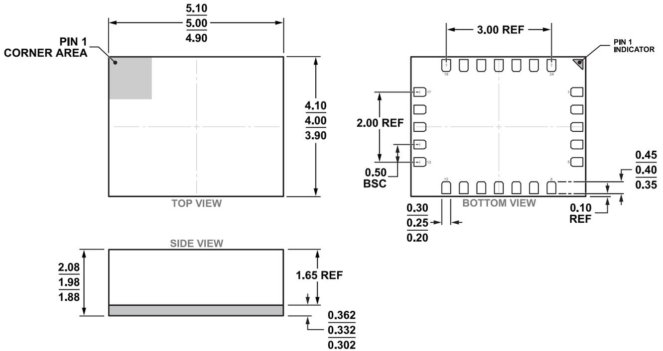
Figure 90. 24-Terminal Land Grid Array [LGA]
