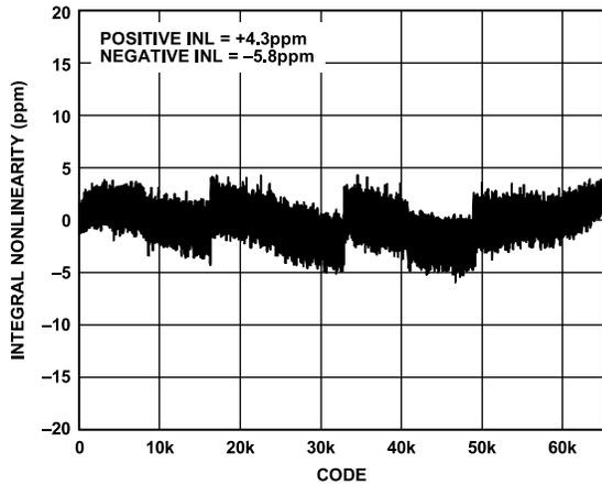
Figure 5. Integral Nonlinearity vs. Code, REF = 5 V
