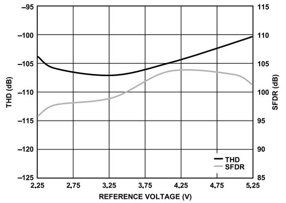
Figure 16. THD and SFDR vs. Reference Voltage
