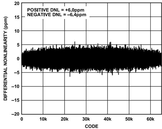
Figure 8. Differential Nonlinearity vs. Code, REF = 5 V
