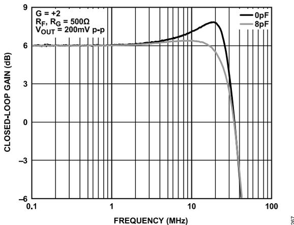
Figure 66. Peaking Mitigation in Small Signal Frequency Response
