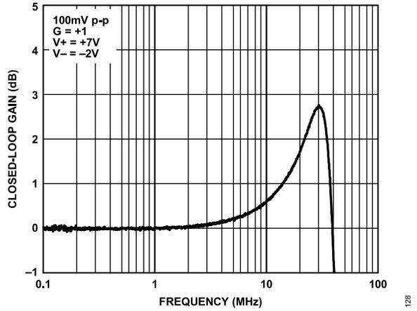
Figure 26. ADC Driver Small Signal 0.1 dB Bandwidth
