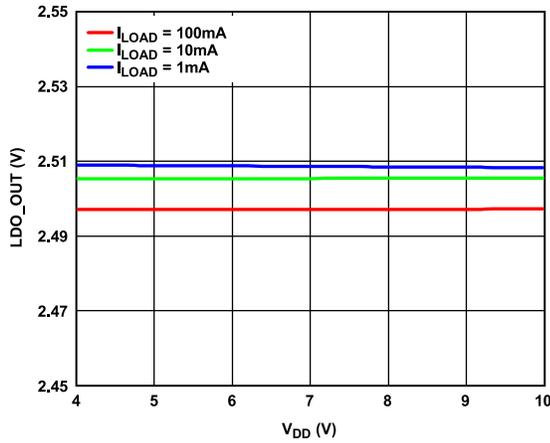
Figure 47. Output Voltage (LDO\_OUT) vs. V<sub>DD</sub>
