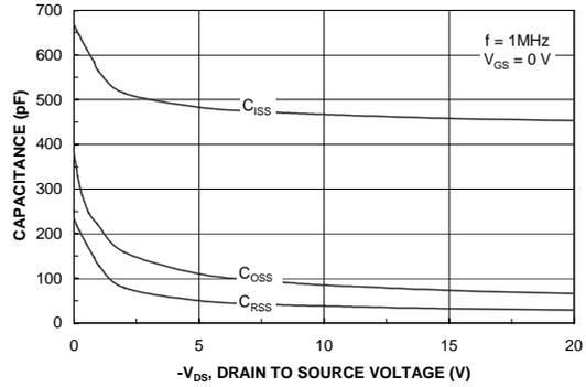
Figure 8. Capacitance Characteristics.
