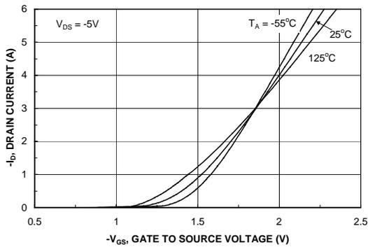
Figure 5. Transfer Characteristics.
