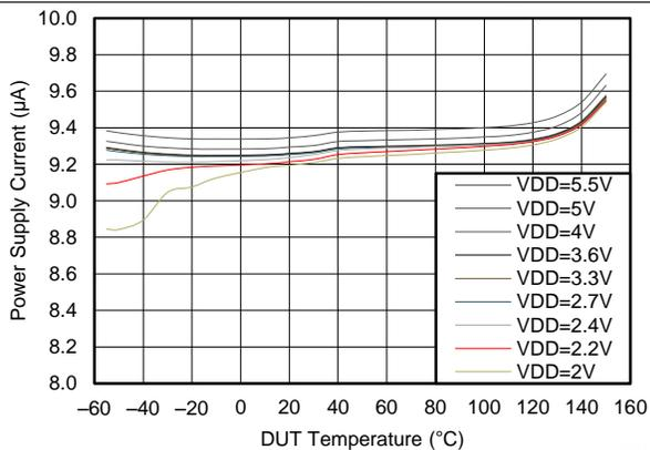
Figure 15. IDD vs Temperature at Various VDD
