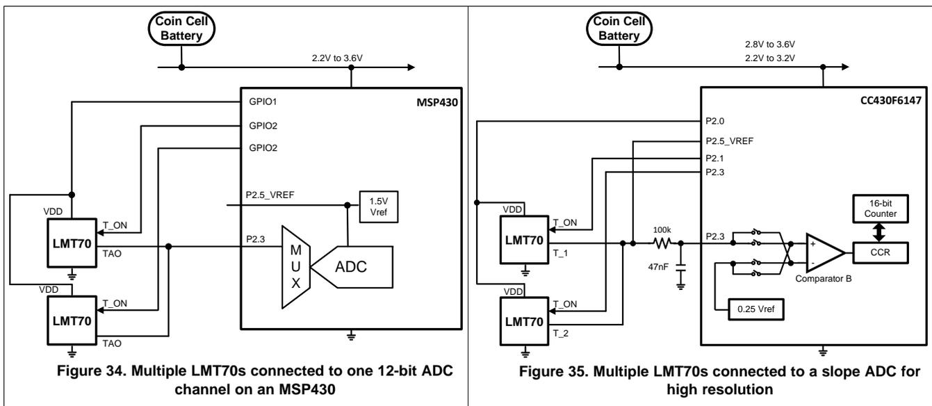
Figure 34. Multiple LMT70s connected to one 12-bit ADC channel on an MSP430
