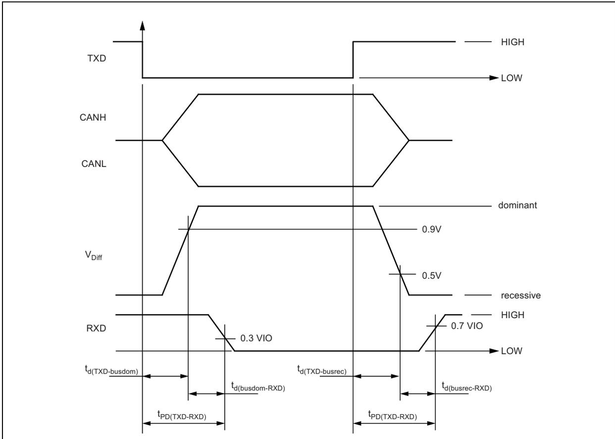
**FIGURE 2-3: CAN TRANSCEIVER TIMING DIAGRAM 2**
