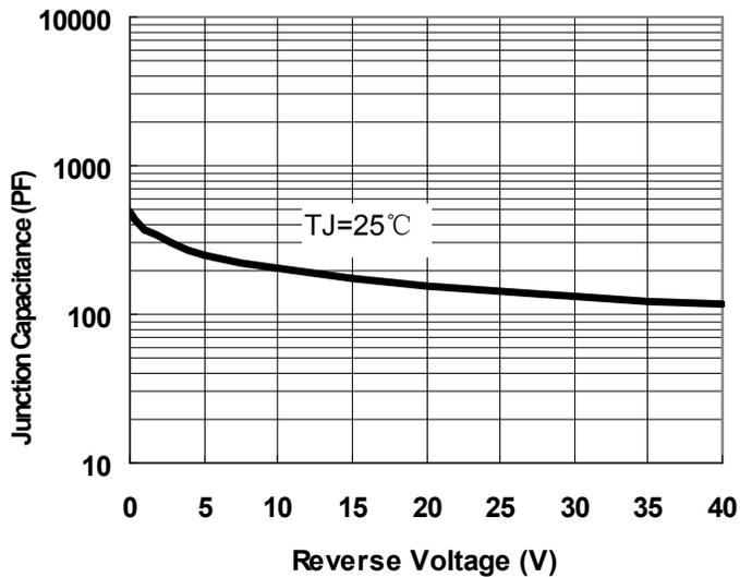
Fig.1-Typical Junction Capacitance
