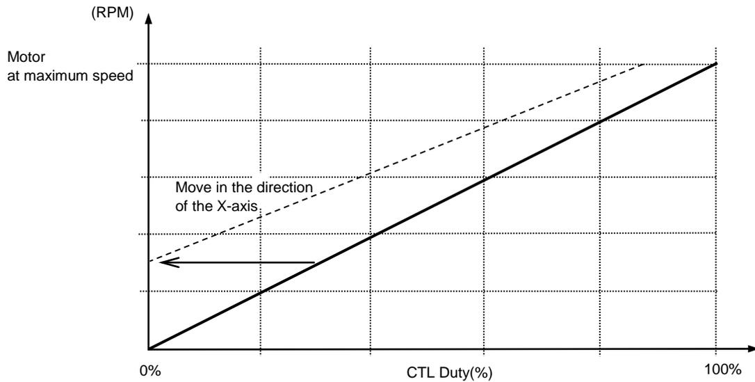
(Example) In the case where the characteristics change from ones with the origin point (0%, 0 rpm) to ones where the speed at a duty ratio of 30% becomes the speed at 0%:
