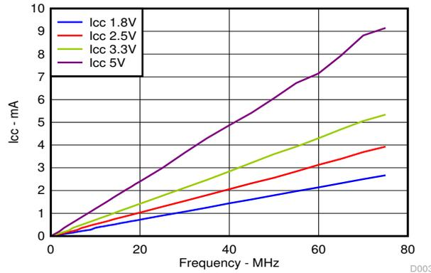
**Figure 9-2. I<sub>CC</sub> vs Frequency**
