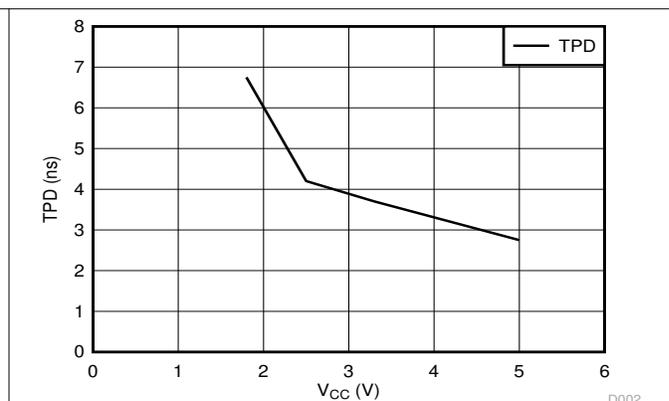
Figure 6-2. TPD Across V<sub>CC</sub> at 25°C
