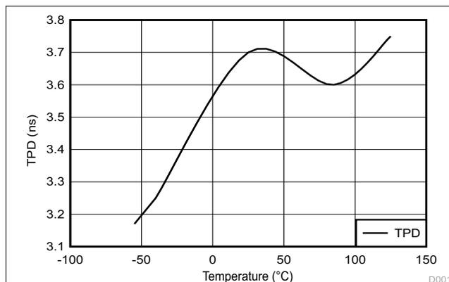
Figure 6-1. TPD Across Temperature at 3.3 V V<sub>CC</sub>
