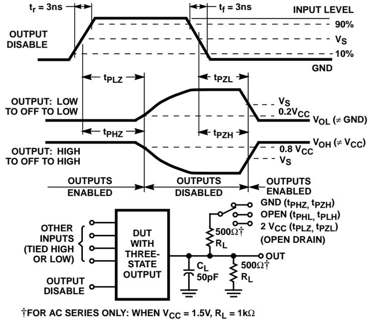
FIGURE 1. THREE-STATE PROPAGATION DELAY WAVEFORMS AND TEST CIRCUIT
