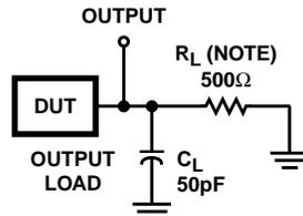
NOTE: For AC Series Only: When  $V_{CC} = 1.5V$ ,  $R_L = 1k\Omega$ .
