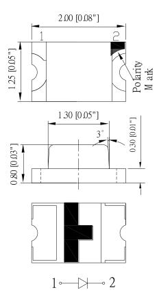
Units: mm / tolerance = +/-0.1mm
