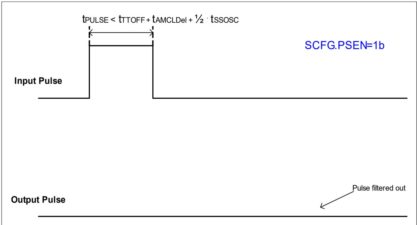
Figure 14 TTOFF: pulse suppressor aborting a turn-on sequence
