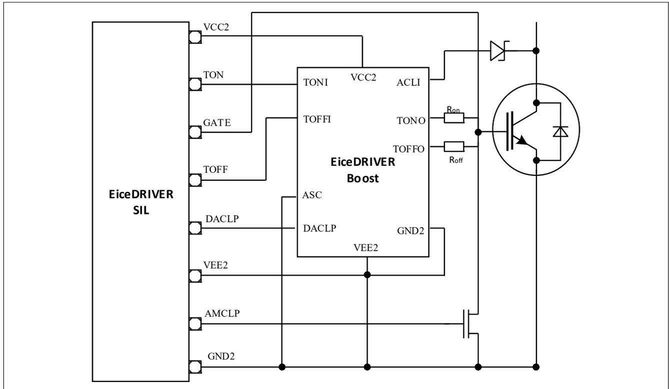
**Figure 12** Output Stage Diagram of Principle
