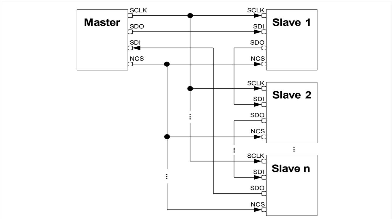
**Figure 7** SPI Daisy Chain Bus Topology
