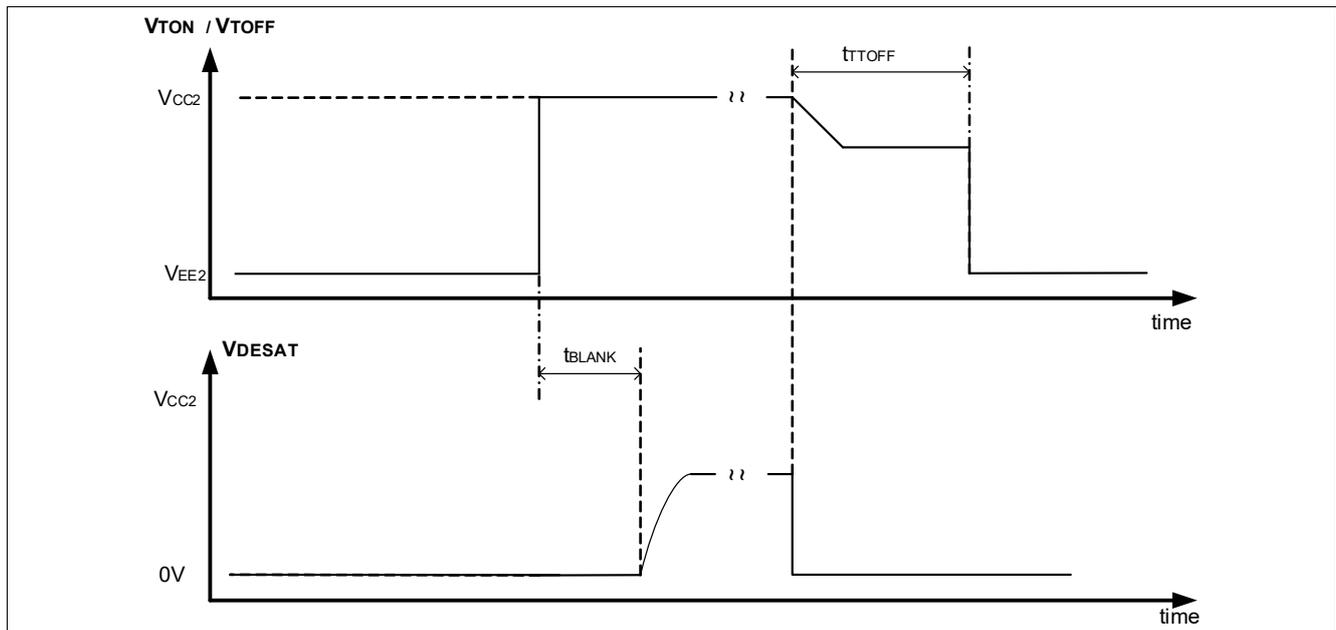
Figure 19 DESAT Operation with DESAT clamping enabled
