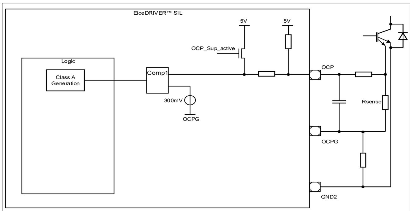
**Figure 20 OCP Function: Principle of Operation**
