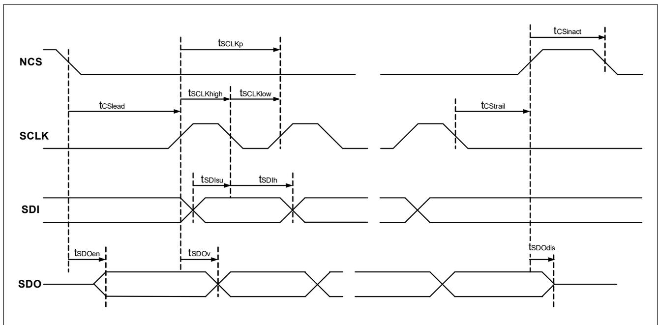
Figure 26 SPI Interface Timing
