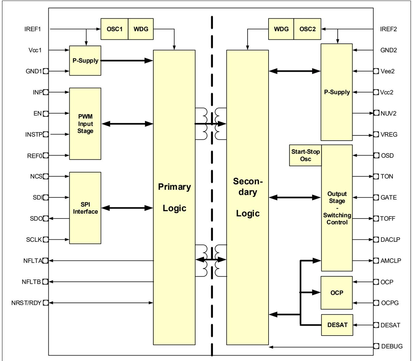
Figure 2 Block Diagram
