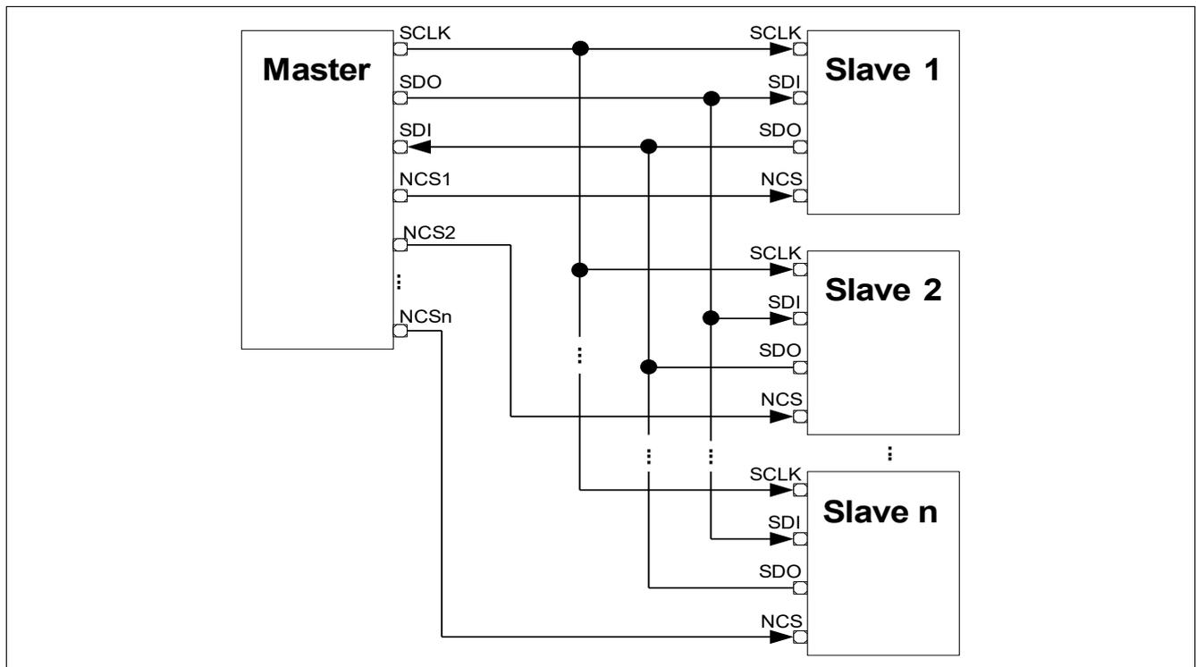
Figure 6 SPI Regular Bus Topology
