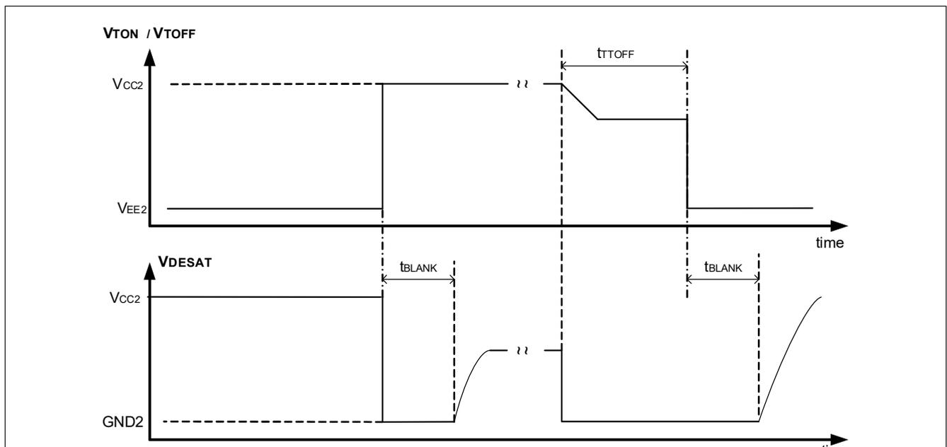
**Figure 18 DESAT Operation**
