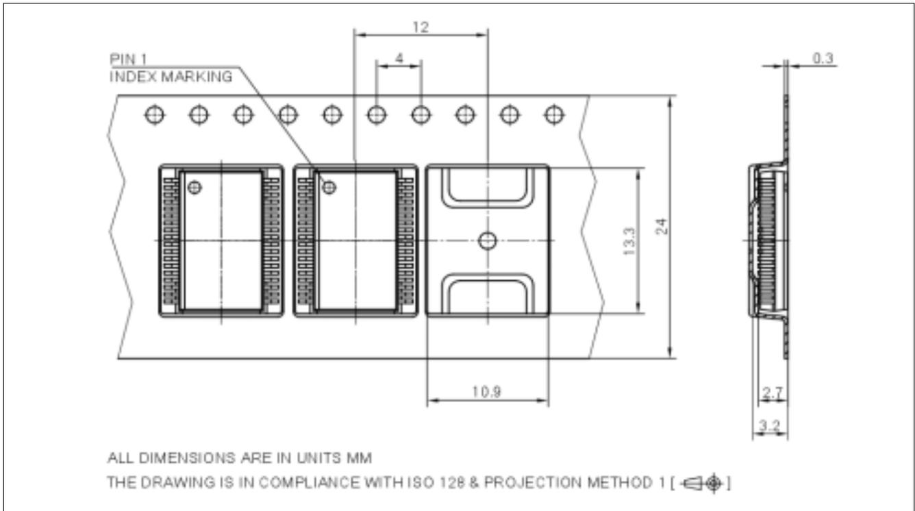
Figure 29 Packing Information (Tape & Reel)
