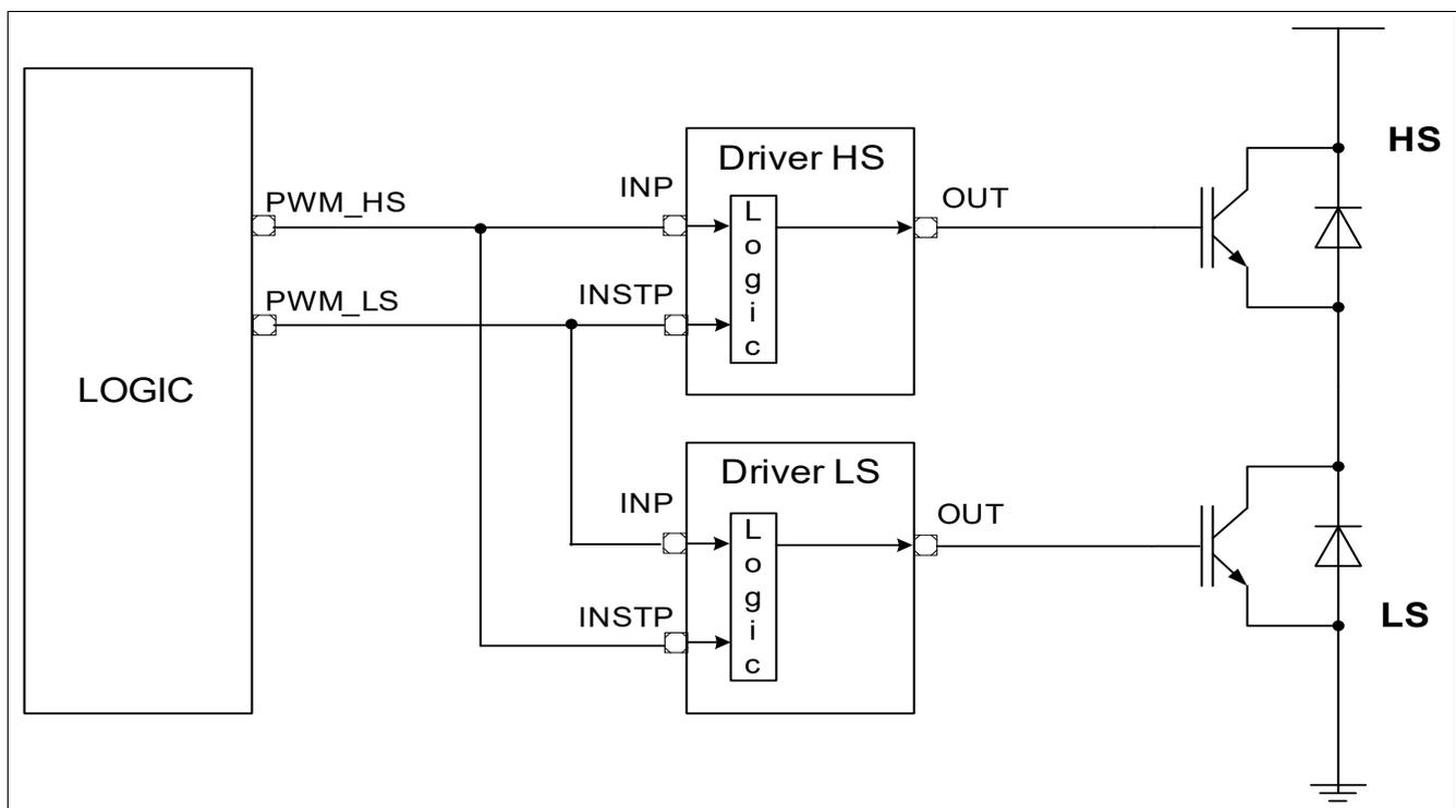
**Figure 22 Shoot Through Protection: Principle of Operation**
