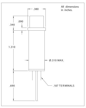
Mounting: Ø.310 MIN., supplied with push-on speednut SN1287.
