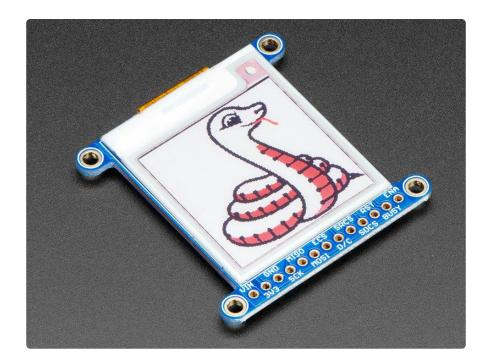
We have multiple tri-color displays. They have black and red ink pixels and a white-ish background. Using our Arduino library, you can create a 'frame buffer' with what pixels you want to have activated and then write that out to the display. Most simple breakouts leave it at that. But if you do the math, using even the smallest 1.54" display: 152 x 152 pixels x 2 colors = 5.7 KBytes. Which won't fit into many microcontroller memories. Heck, even if you do have 32KB of RAM, why waste 6KB?
