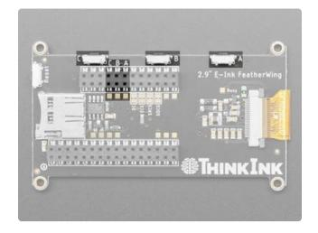
The buttons are connected to Digital Input pins. Pressing the button brings the pin low. There are no pull-up resistors connected, so you will need to enable those in software.
