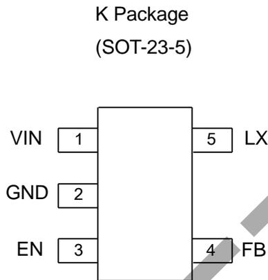
Figure 2. Pin Configuration of AP3410B (Top View)
