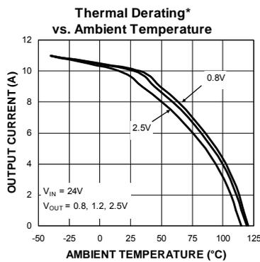
**Die Temperature\*** : The temperature measurement was taken at the hottest point on the MIC26400 case mounted on a 5 square inch 4 layer, 0.62", FR-4 PCB with 2oz finish copper weight per layer, see Thermal Measurement section. Actual results will depend upon the size of the PCB, ambient temperature and proximity to other heat emitting components.
