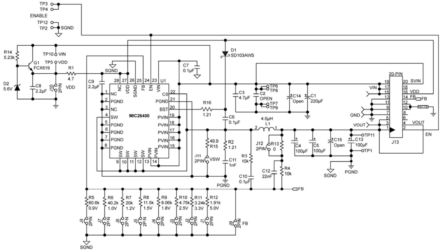
**Figure 8. Schematic of MIC26400 Evaluation Board**
