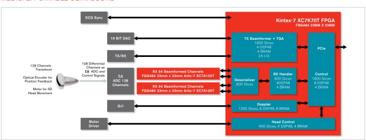
Support for 6.144Gbps CPRI/OBSAI in a low-cost package optionHigh I/O bandwidth and 144GMACS DSP processing power in chip-scale packaging make the Kintex-7 70T FPGA highly effective for both front- and back-end ultrasound processing. Designers can deploy a fully programmable 128-channel ultrasound implementation that scales up to 196 or 256 channels for high-end cart solutions or down to 64 or 32 channels for hand-held solutions.
