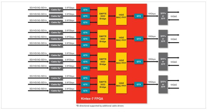
Kintex-7 FPGAs enable cost-effective, low-power bridging of the serial digital interface (SDI) protocol onto IP technology for long-distance WAN transport to link local studios/live events, broadcast facilities, and satellite uplink stations using standard IP networks.
