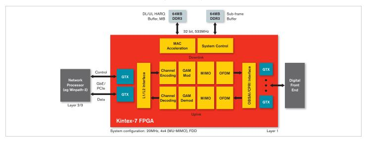
Kintex-7 FPGAs offer the best price-performance so designers can meet stringent latency requirements for LTE baseband processing in a common platform.
