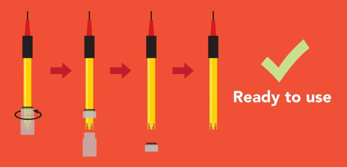
2 During shipment the air bubble in the probes stem may move into the bulb area. If bubbles are seen in the bulb area, hold the probe by its top cap and shake downward as done with a clinical thermometer.
