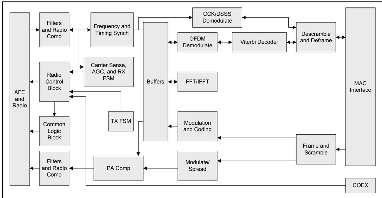
The PHY is capable of fully calibrating the RF front end to extract the highest performance. On power-up, the PHY performs a full suite of calibration to correct for IQ mismatch and local oscillator leakage. The PHY also performs periodic calibration to compensate for any temperature related drift thus maintaining high-performance over time. A closed loop transmit control algorithm maintains the output power to required level with capability control TX power on a per packet basis.
