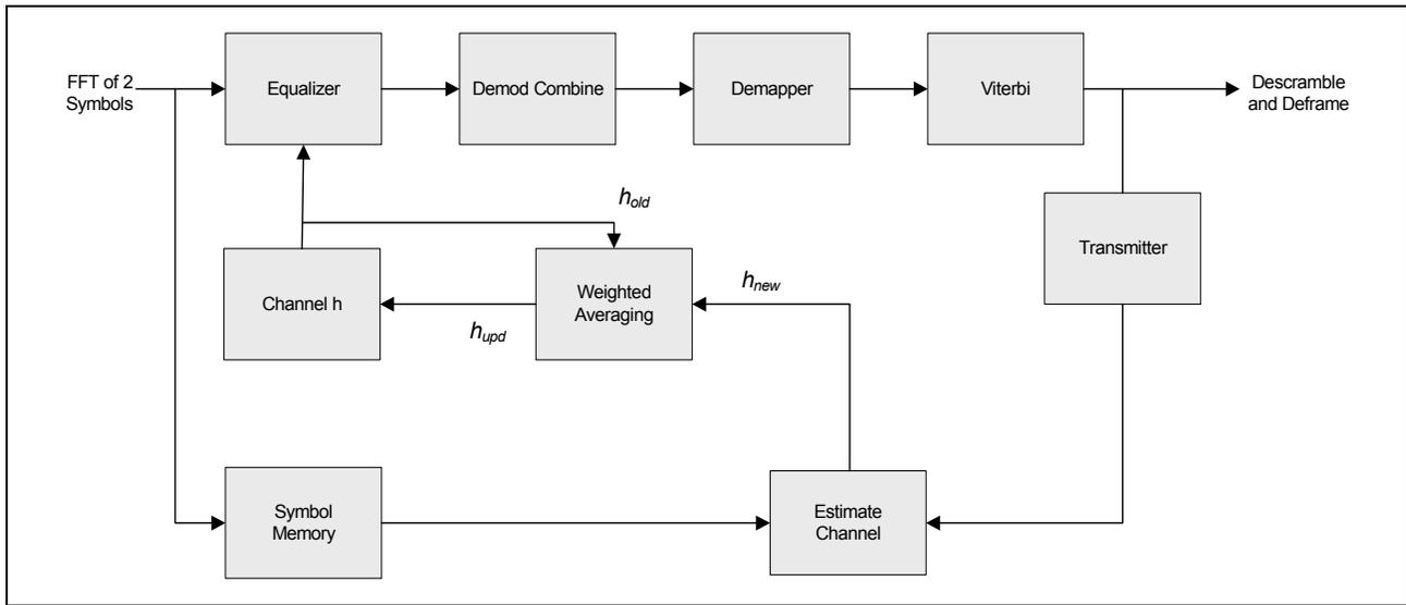
In STBC mode, symbols are processed in pairs. Equalized output symbols are linearly combined and decoded. Channel estimate is refined on every pair of symbols using the received symbols and reconstructed symbols.
