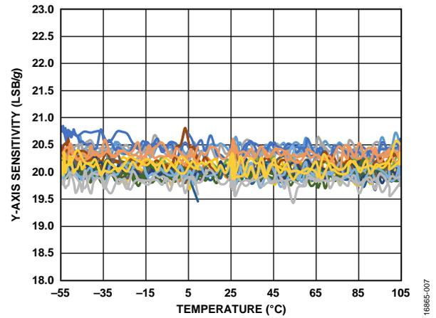
Figure 7. Y-Axis Sensitivity vs. Temperature, 15 Devices Soldered to PCB,  $V_S = 2.5\text{ V}$
