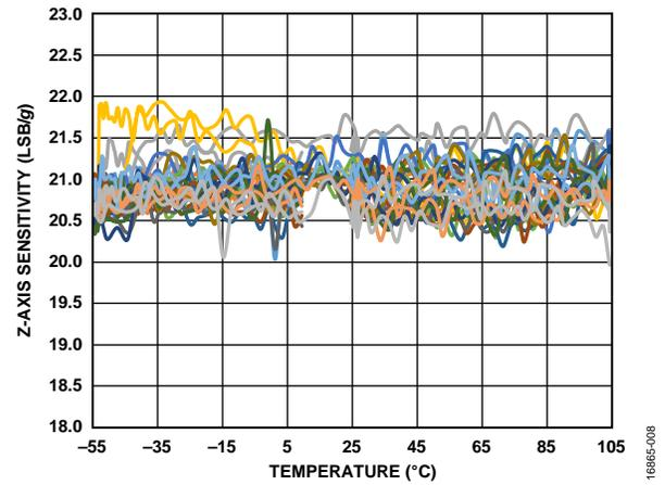
Figure 8. Z-Axis Sensitivity vs. Temperature, 15 Devices Soldered to PCB,  $V_S = 2.5\text{ V}$
