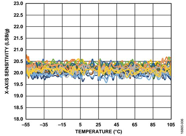
Figure 6. X-Axis Sensitivity vs. Temperature, 15 Devices Soldered to PCB,  $V_S = 2.5\text{ V}$
