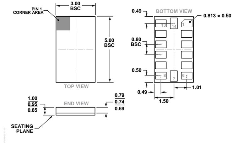
Figure 9. 14-Terminal Land Grid Array [LGA]
