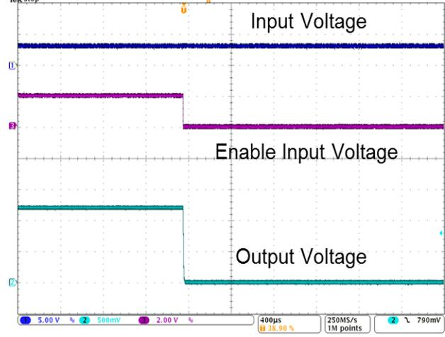
$V_{IN} = 3.3V, V_{OUT} = 1.2V, I_{OUT} = 150mA, C_{IN} = C_{OUT} = 0.1\mu F$
