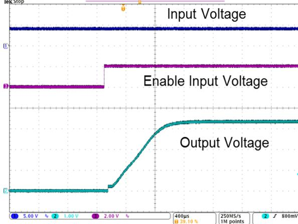
$V_{IN} = 4.3V, V_{OUT} = 3.3V, I_{OUT} = 0mA, C_{IN} = C_{OUT} = 0.1\mu F$
