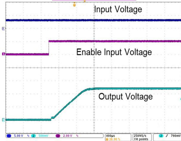
$V_{IN} = 3.3V, V_{OUT} = 1.2V, I_{OUT} = 150mA, C_{IN} = C_{OUT} = 0.1\mu F$
