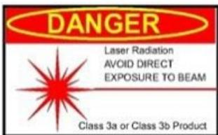
The VCSEL is a class 3b laser and is to be treated as a potential eye hazard. Due to the size of the component, the applicable warning logotype, aperture label, and certification/identification label can not be placed on the component itself.
