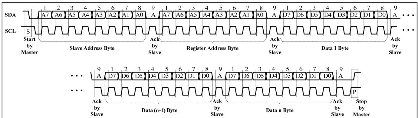
**Figure 5** Writing to IS31FL3195 (Automatic Address Increment)
