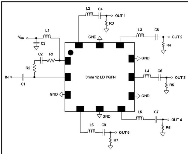
8. The exposed pad centered on the package bottom must be connected to ground for RF, DC and thermal considerations.
