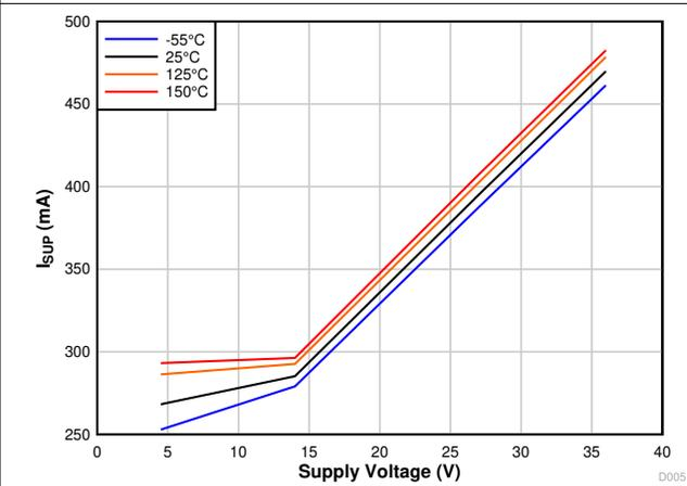
Figure 7-4.  $I_{SUP}$  Recessive vs  $V_{SUP}$  and Temperature
