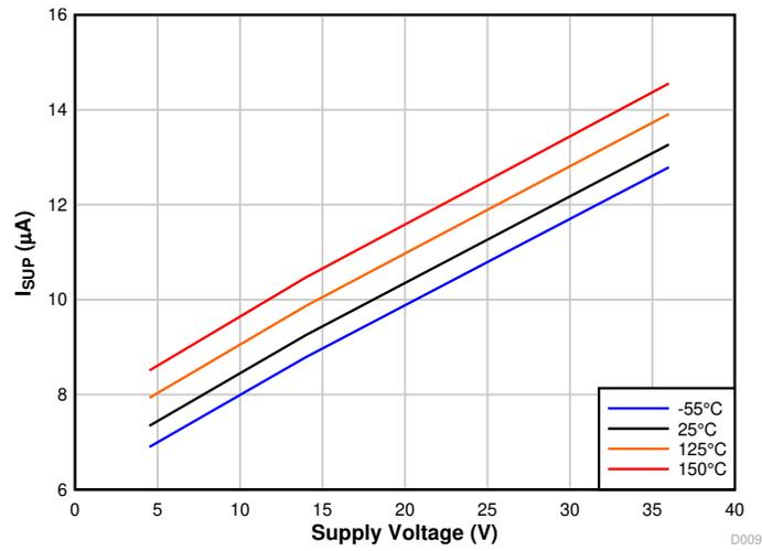
Figure 7-7. Sleep Mode I<sub>SUP</sub> vs V<sub>SUP</sub> and Temperature
