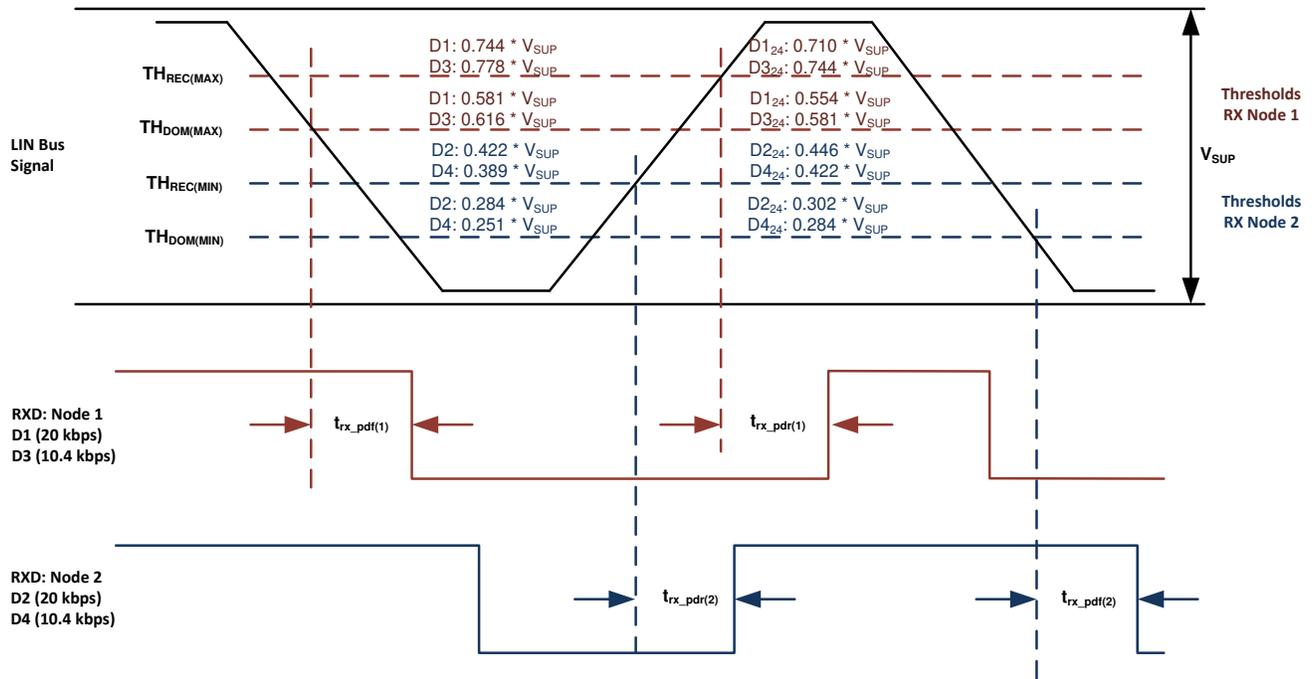
Figure 8-14. Propagation Delay
