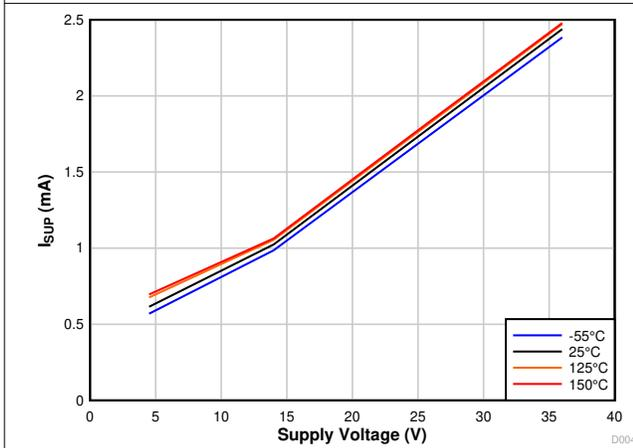
Figure 7-3.  $I_{SUP}$  Dominant vs  $V_{SUP}$  and Temperature
