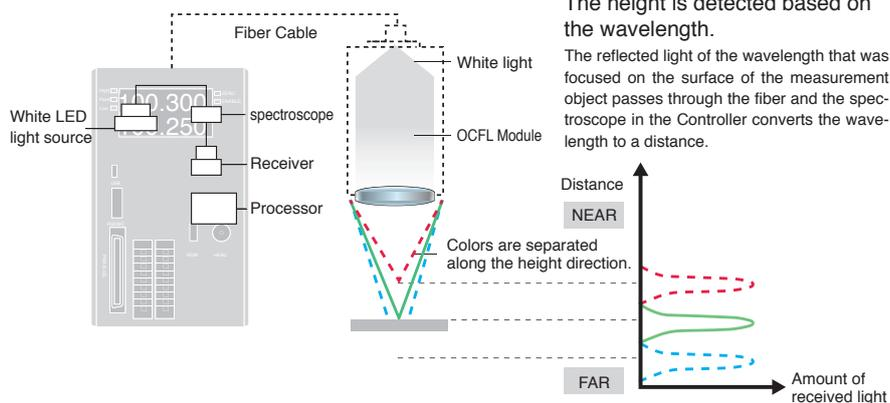
The height is detected based on the wavelength.
