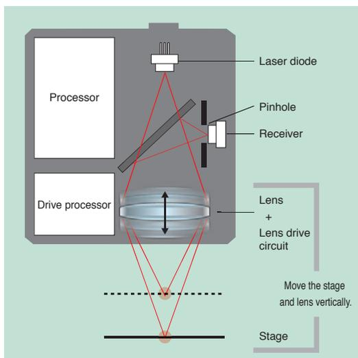
In a normal confocal model, a stage and lens are driven vertically to change the focal point. This requires a more complex structure, and the large number of parts interferes with downsizing. The use of a laser beam increases the chances of interference, and the received light waveform can be disrupted by the surface conditions within the small spot on the measurement object.
