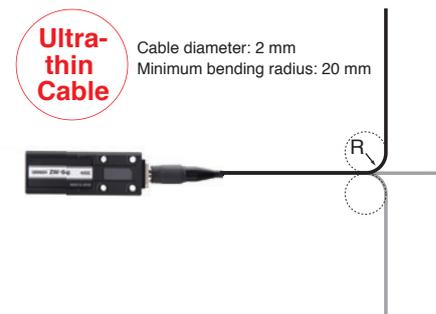
\*Cable was tested with OMRON's bending test consisting of 2,000,000 bends to a 70-mm bending radius and 1,000,000 bends to a 20-mm bending radius.
