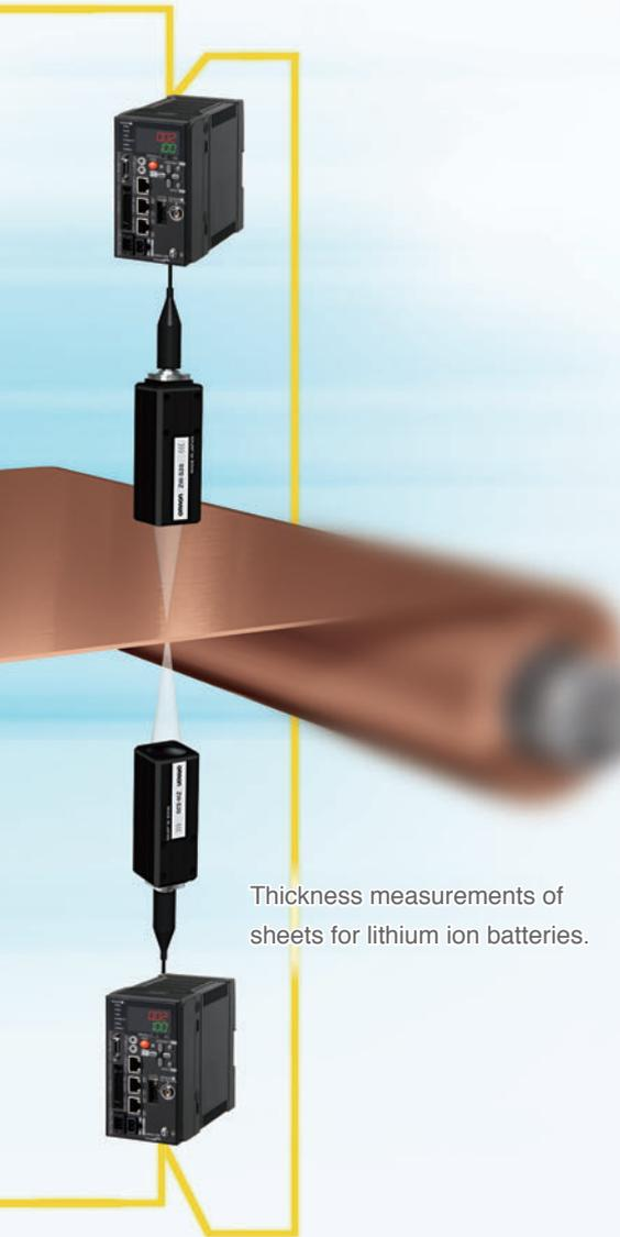
Thickness measurements of sheets for lithium ion batteries.
