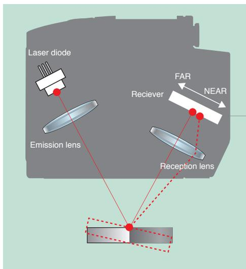
Triangulation measures the height of an object based on the position of the spot on a receiver (CCD or CMOS). The peak, center of gravity, and other features are calculated from the received light waveform to reduce error, but in principle, the received waveform is offset or disrupted due to differences in materials or inclination. This results in measurement error.
