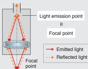
The height is calculated from the position at which the reflected light was received.
